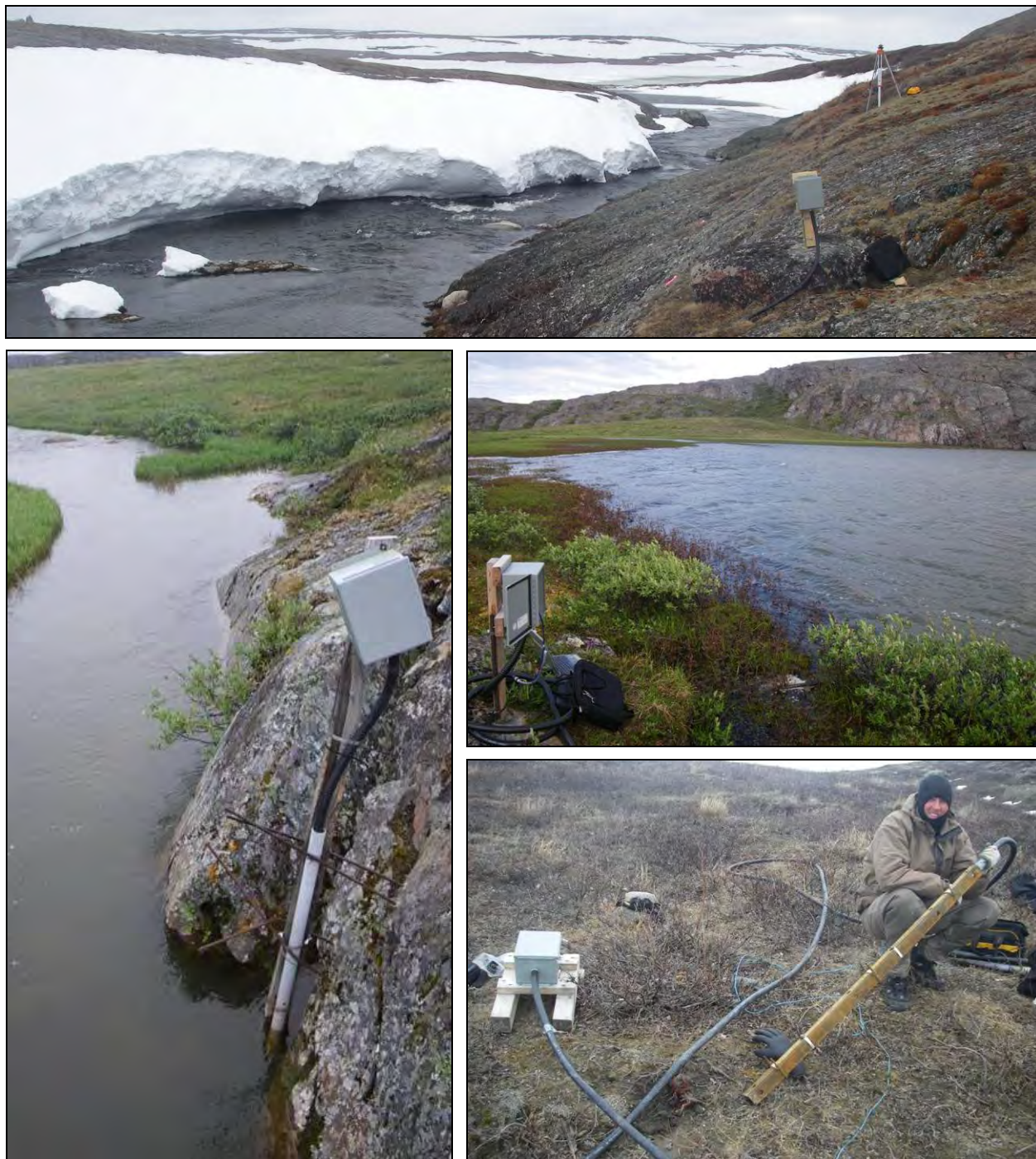
Plate 3.1-1. Photographs illustrating hydrometric station design.
