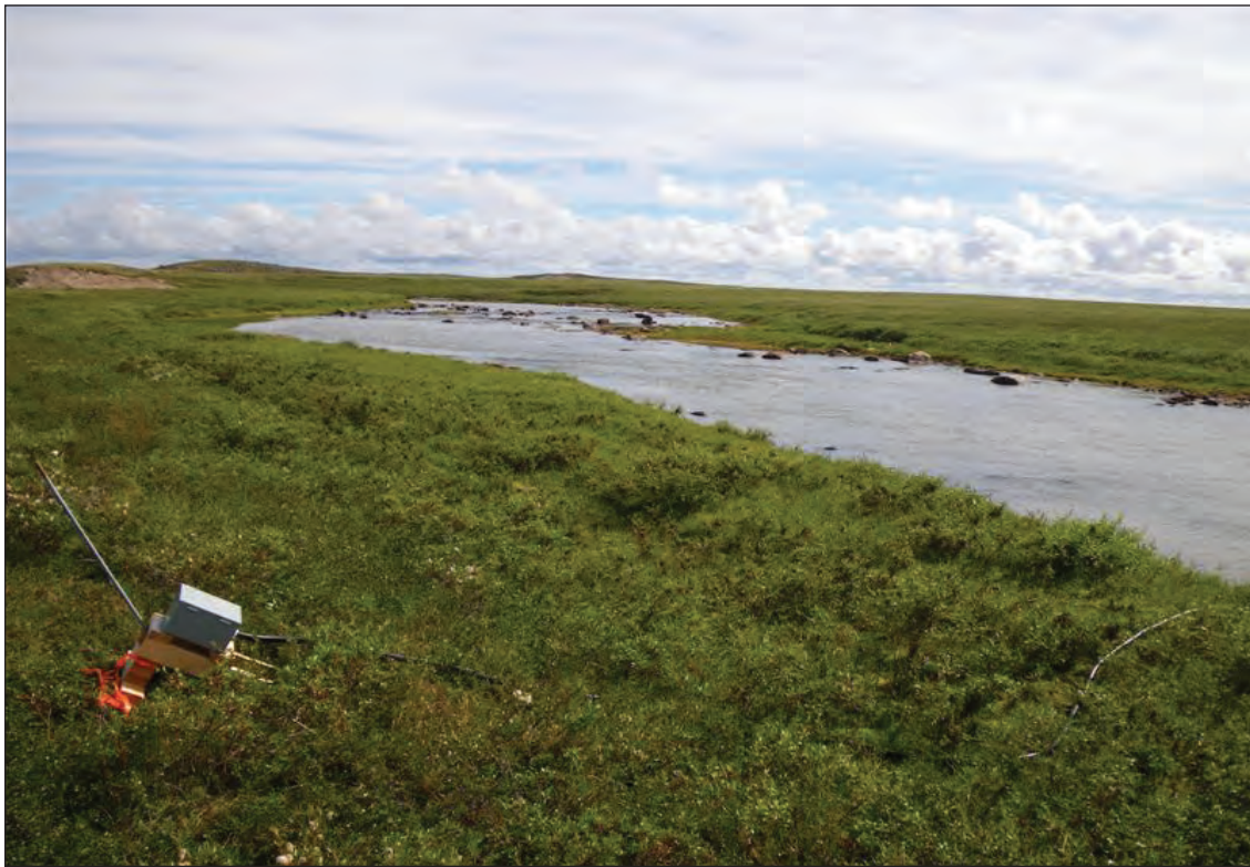
Photograph taken facing upstream (south east) from the hydrometric station East Aimao Hydro, located on a relatively narrow section along the banks of the eastern tributary of Aimaokatalok Lake. Note how the flow is confined to the main channel during low to medium flow conditions. During high flow conditions the channel overflows into grass-covered flood terraces that can be observed alongside the right bank on the background in the photograph. Photograph taken on July 20, 2010.
