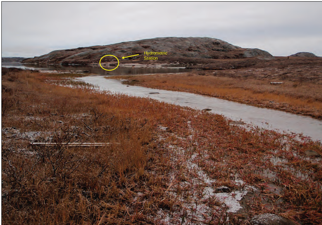
Patch Lake outlet channel, looking upstream (west) toward the hydrometric station Patch-Hydro. The flow is confined by the channel at low and medium flow conditions. During high flow conditions the channel overflows a flood terrace overgrown with vegetation located along the left bank. Photograph taken on October 1st, 2010.
