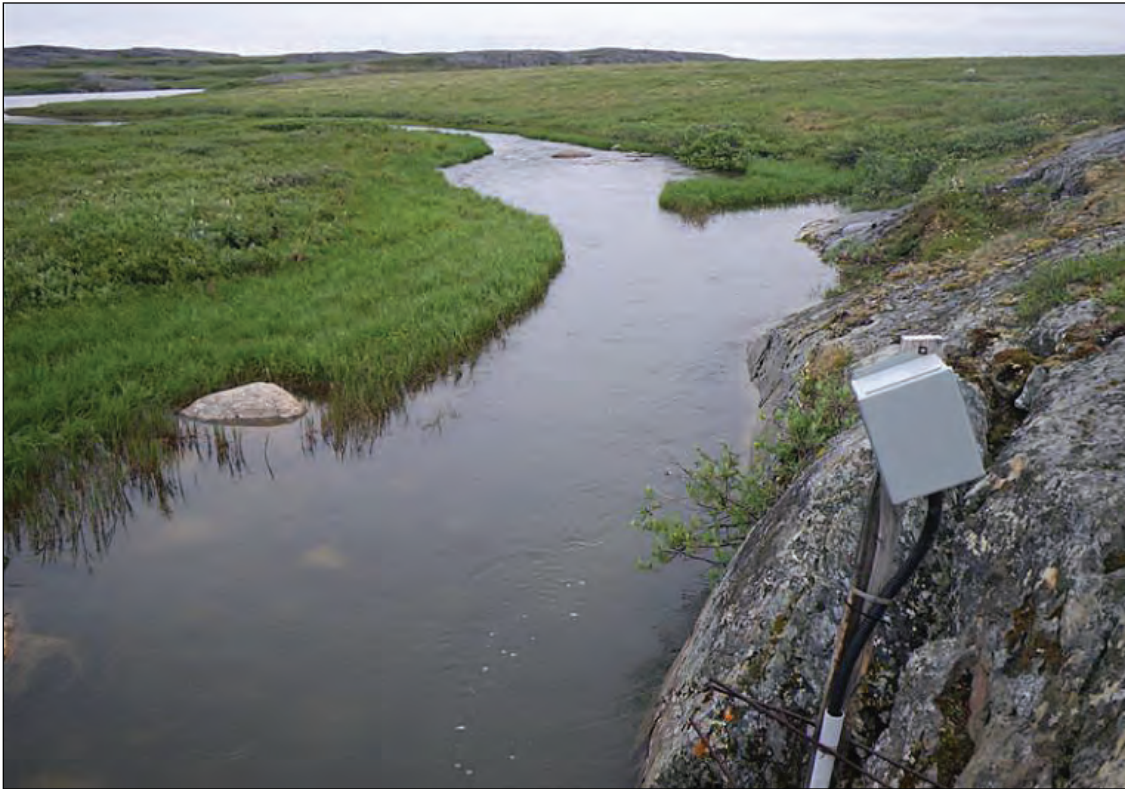
Ogama-Hydro, looking upstream (south) from the hydrometric station toward the outlet of Ogama Lake. Note how the flow is confined to the main channel by a bedrock outcrop along the left bank. However, during high flow conditions the channel can overflow onto a flood terrace located along the right bank. Photograph taken on July 16th, 2010.
