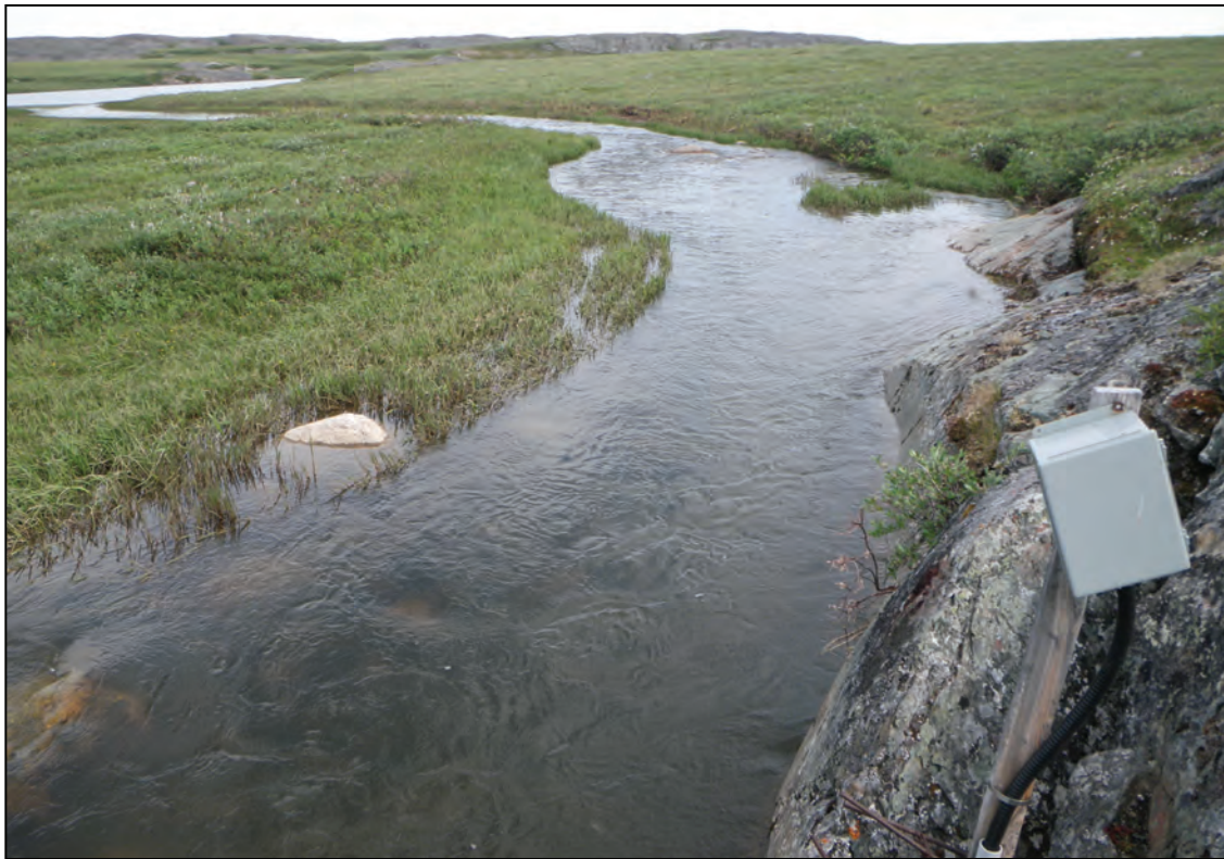
Ogama outflow facing upstream and south towards Ogama Lake at the hydrometric station. Note the bedrock outcrop along the left bank that confines flow in the main channel. During high flow conditions the channel overflows onto the flood terrace located along the right bank. Photograph taken on July 21, 2011.
