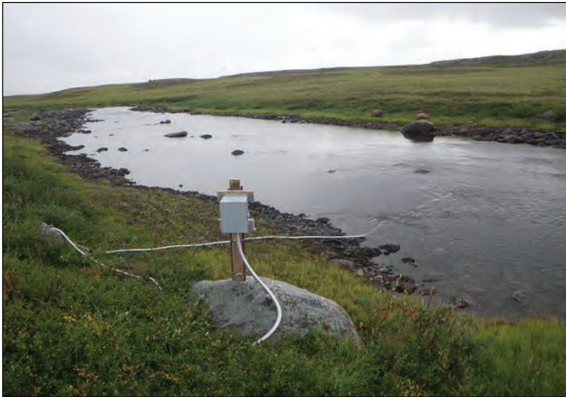
Aimaokatalak inflow facing upstream and south at the hydrometric station. Note how the flow is confined to the main channel during low to medium flow conditions. During high flow conditions the channel overflows into grass-covered flood terraces that can be observed alongside the right bank on the background in the photograph. Photograph taken on August 20, 2011.
