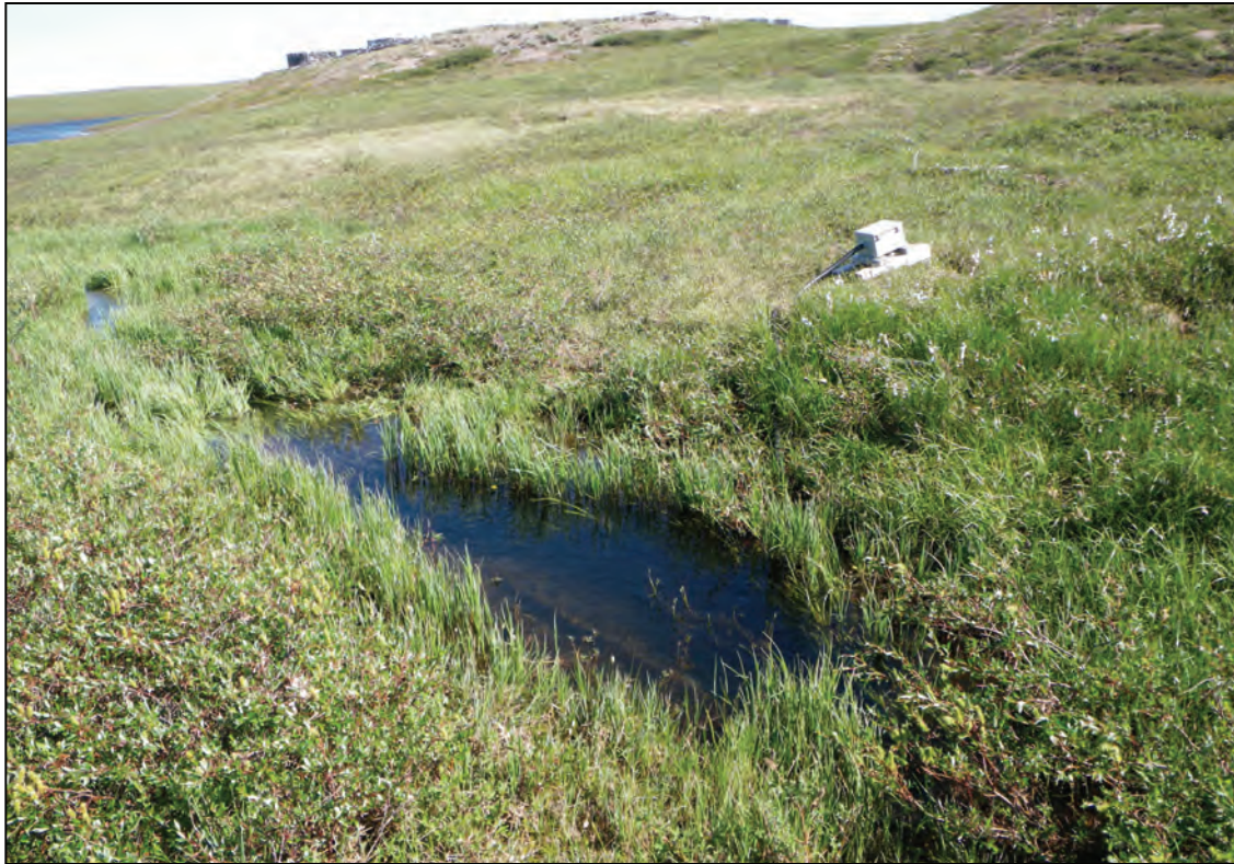
Stickleback Lake outflow facing downstream and northeast at the hydrometric station. Note how the channel is very narrow and the flow is well confined to the main channel during low to medium flow conditions. During high flow conditions the channel overflows into surrounding grass-covered flood terrace. Photograph taken on July 19, 2011.
