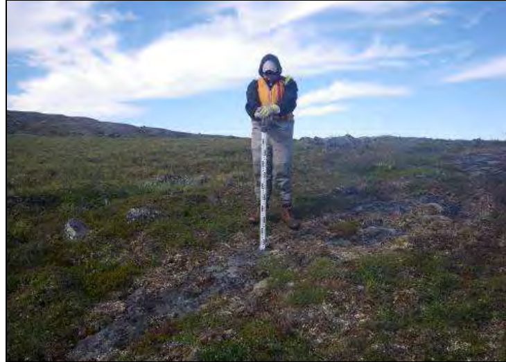
Holding surveyors rod for elevation measurement
