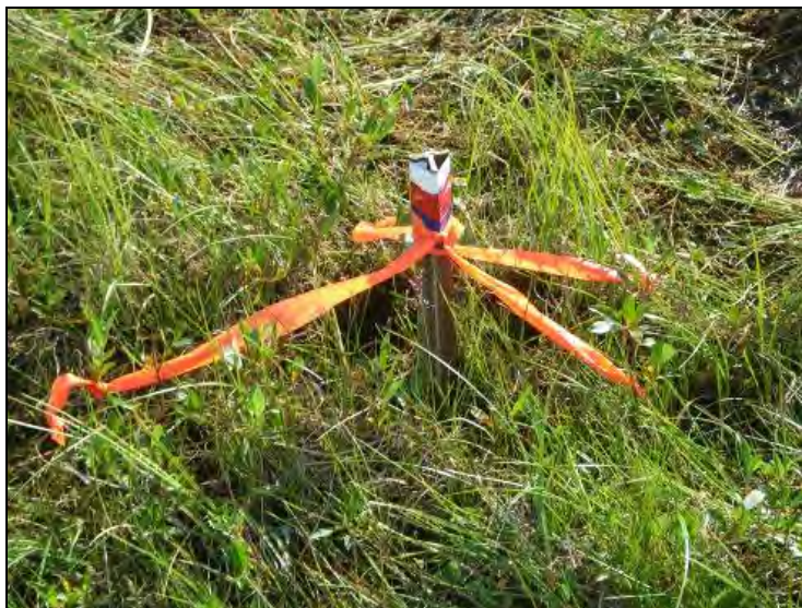
Benchmark installed along shoreline
