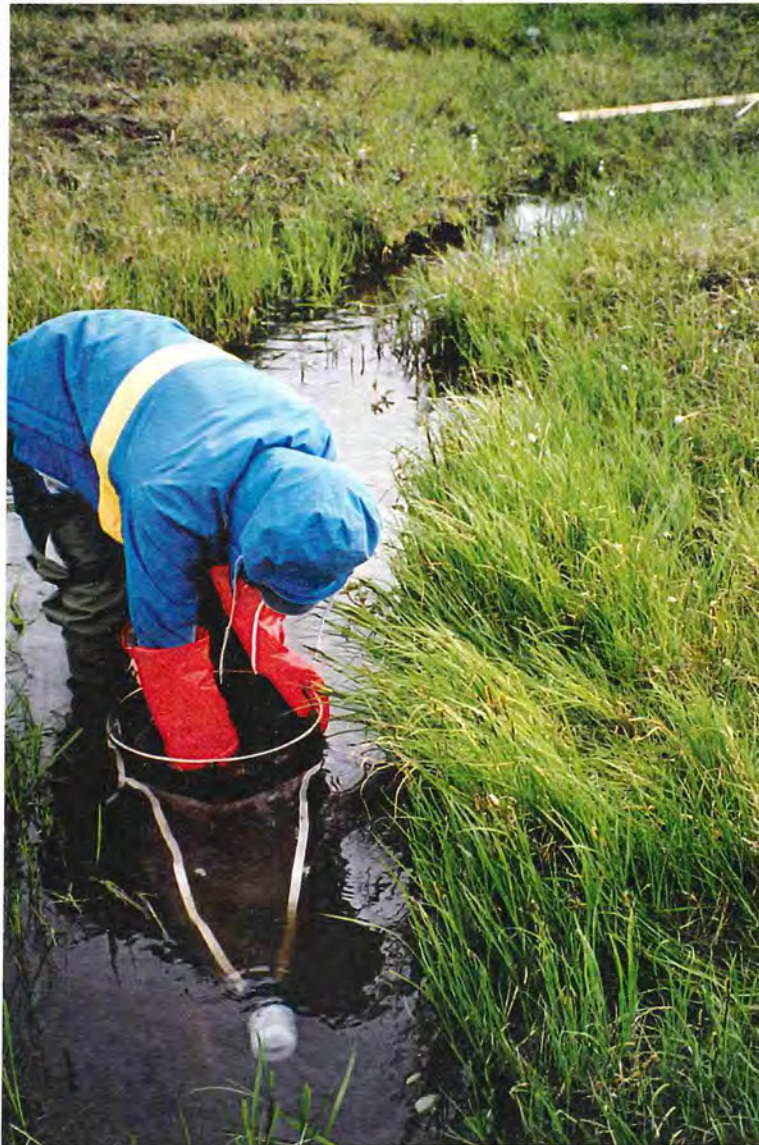
Plate 2-6: A Hess sampler was used at stream sites to sample benthic invertebrates.
