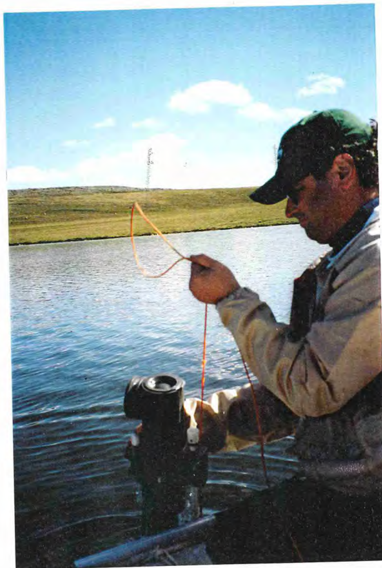
Plate 2-5: A Go-Flo sampling bottle was used in lakes to collect water samples for chemical and biological analyses.
