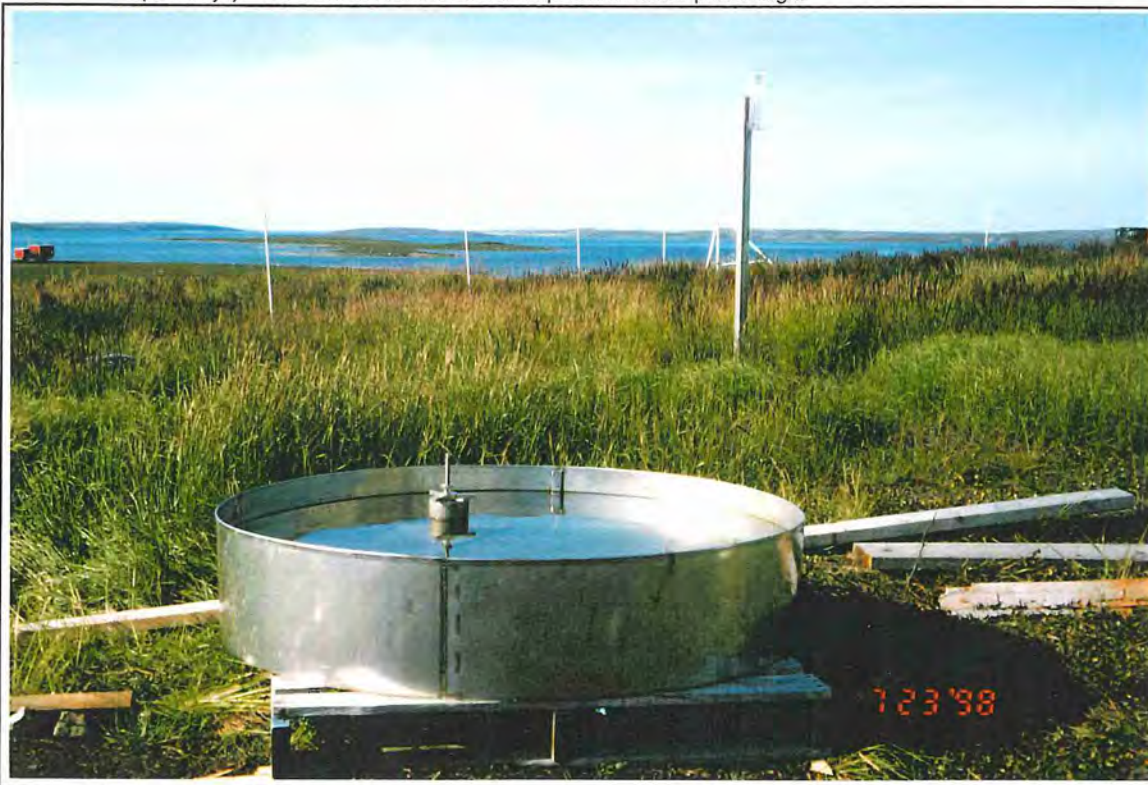
Plate 2.1-2 A Class A Evaporation pan was installed at the Boston exploration camp to monitor evaporation. The hook gauge and stilling well can be seen in the middle of the pan. The instrument required daily supervision and was only read when the camp was occupied. Daily rainfall data from the manual rain gauge (behind and to the right of the pan) are also required for evaporation calculations.
