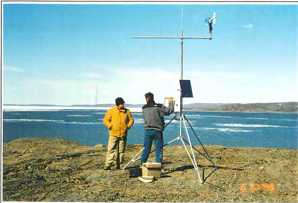
Plate 2.1-1 The automated weather station installed at Roberts Bay was in operation from June 3 to December 1, 1998 (181 days). The wind data will be used for potential future port design.
