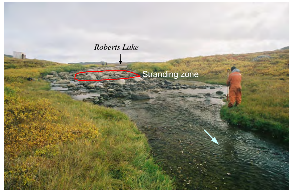
Plate 16 Roberts Outflow, 1 September 2002. Survey measurements of the boulder garden area to determine stream gradient.
