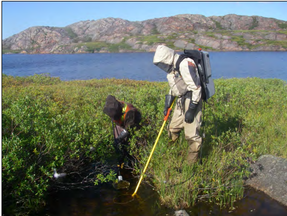
Plate 2.2-2. Backpack electrofishing gear used to assess the fish communities in streams, Hope Bay Belt Project, 2010.
