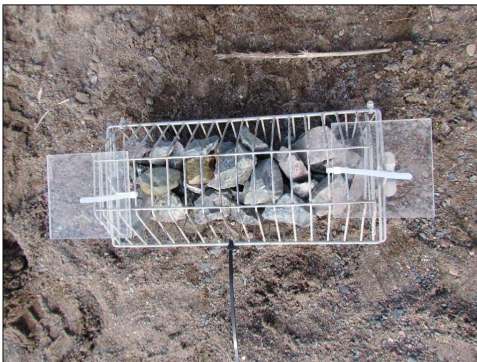
Plate 2.2-1. Rock Trap benthic macroinvertebrate sampler deployed in Windy Lake on July 11, 2013. Two Plexiglas® plates for collecting periphyton were attached horizontally at each end.
