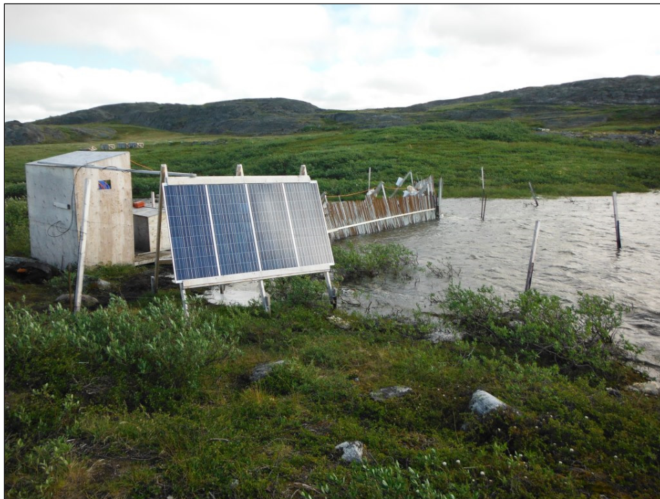
Plate 3.3-1. Solar panels providing power to the Vaki Riverwatcher upstream of the boulder garden, July 21, 2015.
