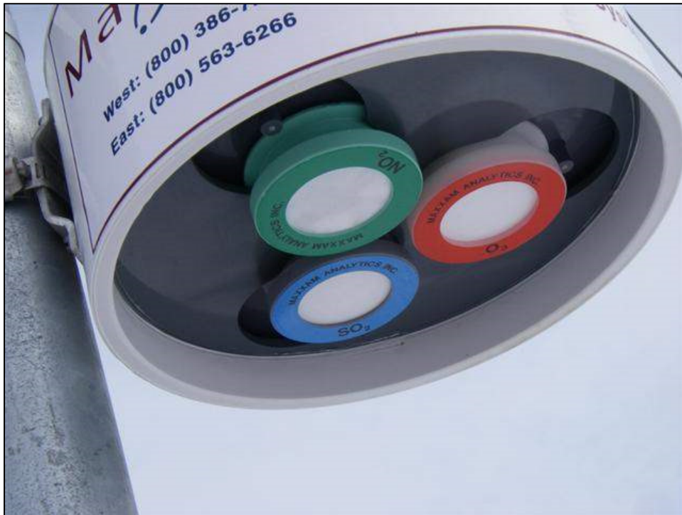
Plate 2.2-4. A Passive Air Sampling System (PASS), monitoring \text{SO}_2 , \text{NO}_2 and \text{O}_3 .
