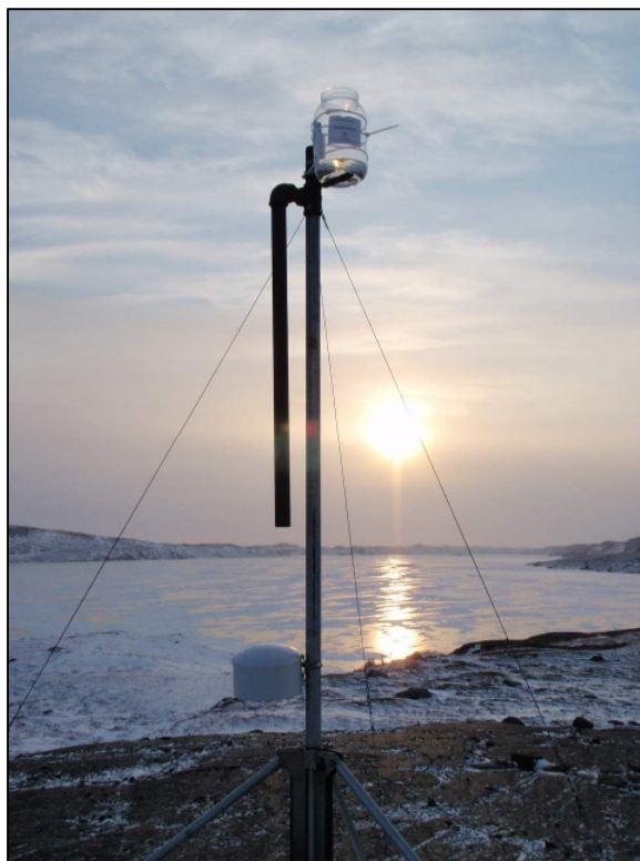
Plate 2.2-3. Dustfall station DFA1 (Alberta method). October 2011.
