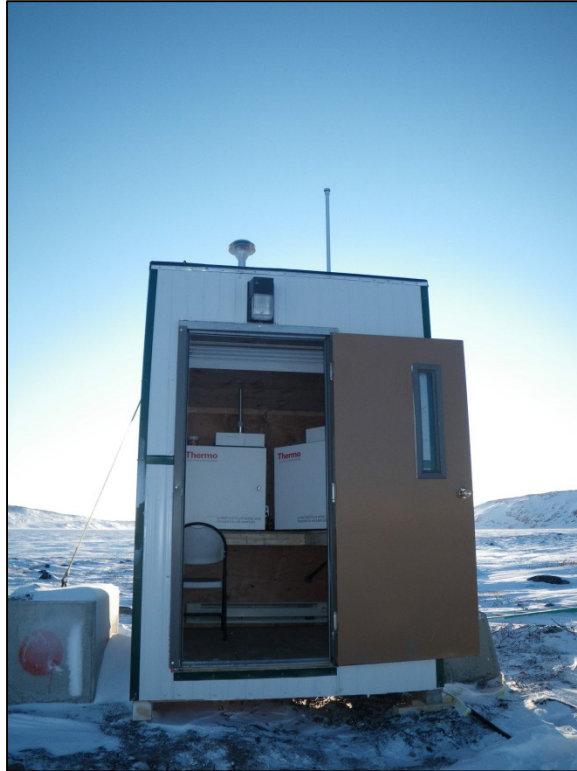
Plate 2.2-1. Partisol samplers inside the temperature controlled shelter. February 2012.
