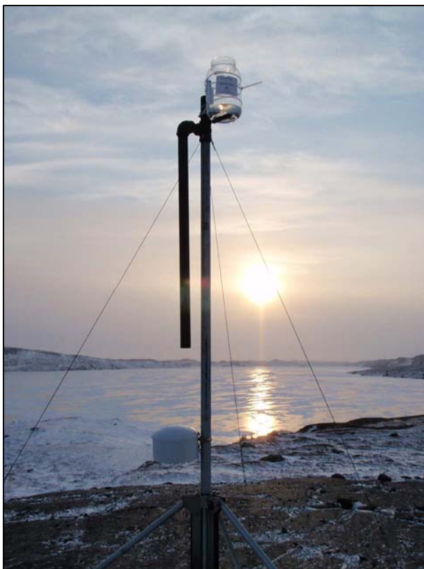
Plate 2.3-3. Dustfall station DFA1 (Alberta method). October 2011.
