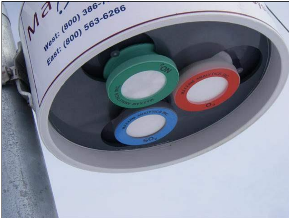
Plate 2.3-4. A Passive Air Sampling System (PASS), monitoring \text{SO}_2 , \text{NO}_2 and \text{O}_3 .
