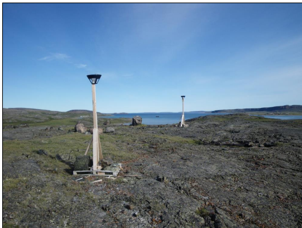
Plate 2.3-2. Dustfall station DF1 (ASTM method). July 2010.
