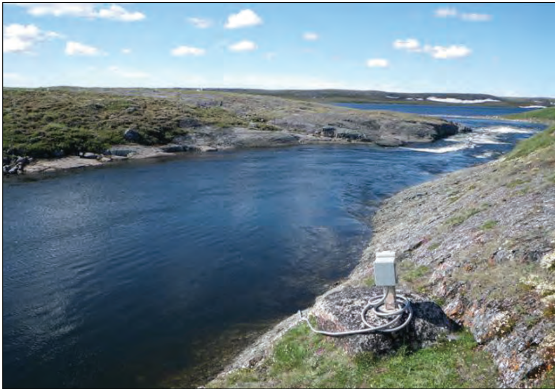
Aimaokatalak Lake outflow facing downstream and west from the hydrometric station. Note how the flow is confined to the main channel the control section can be observed where water becomes more turbulent. Aimaokatalak Lake outflow flows into the Koignuk River shown in the background of the photograph. Photograph taken on July 17, 2011.
