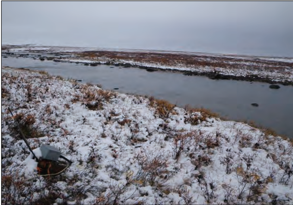
East Aimaokatalak outflow facing upstream and southeast at the hydrometric station. The hydrometric station is located on a relatively narrow section along the banks of the eastern tributary of Aimaokatalok Lake. Note how the flow is confined to the main channel during low to medium flow conditions. During high flow conditions the channel overflows into grass-covered flood terraces that can be observed alongside the right bank on the background in the photograph. Photograph taken on September 19, 2011.
