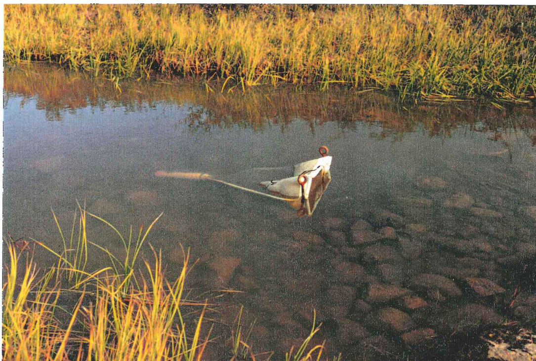
Plate 3-4: A larval drift net sampler was set for 24 hr in Trout Creek, where some flow was recorded, but low flow combined with low water levels hampered sampling efficiency (water depth <15 cm).
