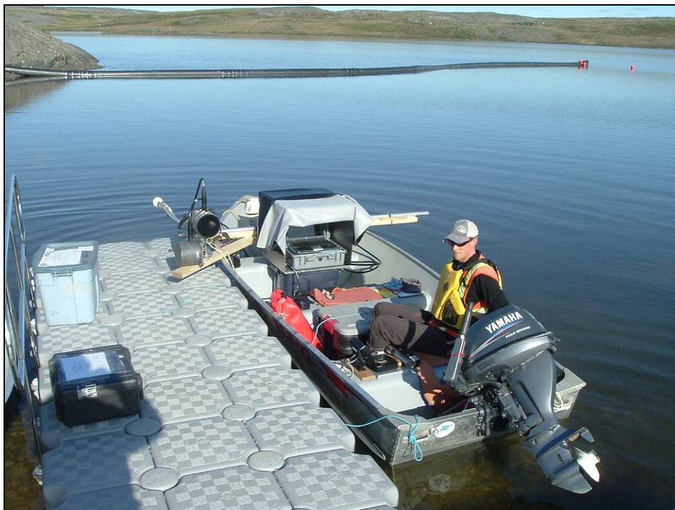
Plate 2.1-1. Hydroacoustics system used to conduct substrate classification and fish abundance estimates at Doris and Patch lakes, Hope Bay Belt Project, 2009.
