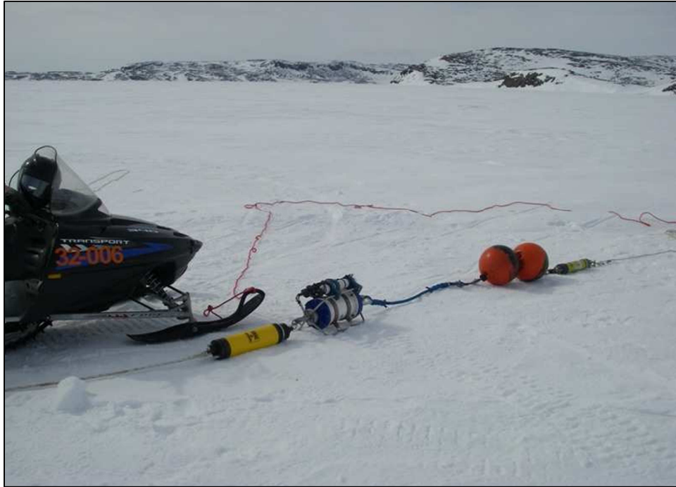
Plate 2.4-2. Photograph of the bottom taut-line mooring in April 2011, before deployment at 85 m site at mouth of Roberts Bay.
