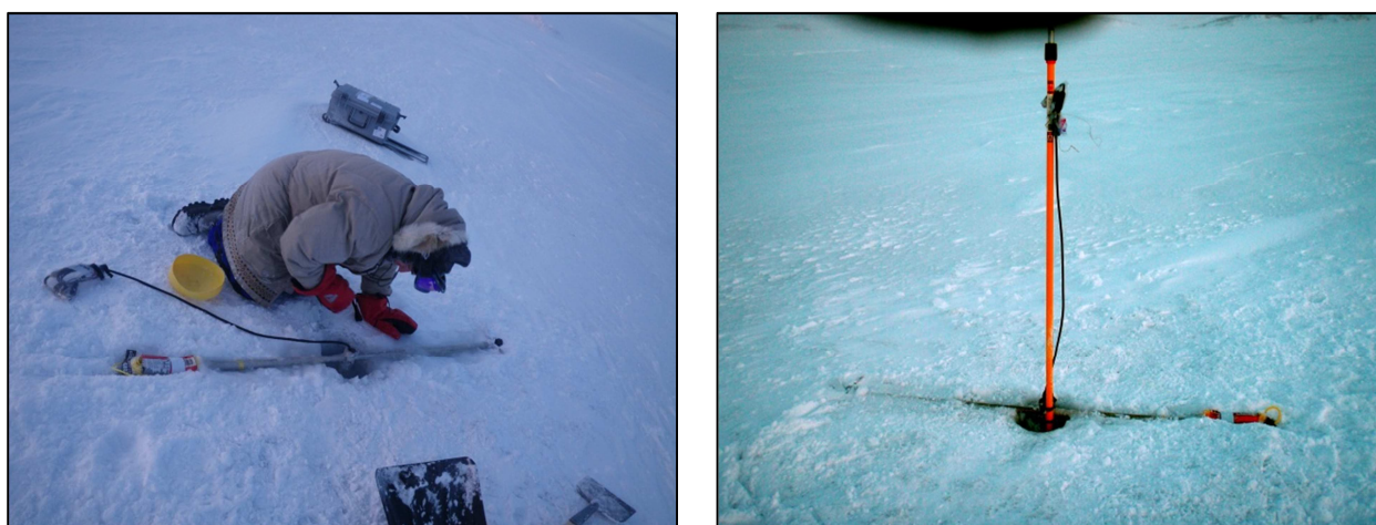
Plate 2.4-1. Deployment of the ice-mounted 300 kHz ADCP in February 2011. The ADCP was downward looking, at a depth of 3.8 m from the ice surface.
