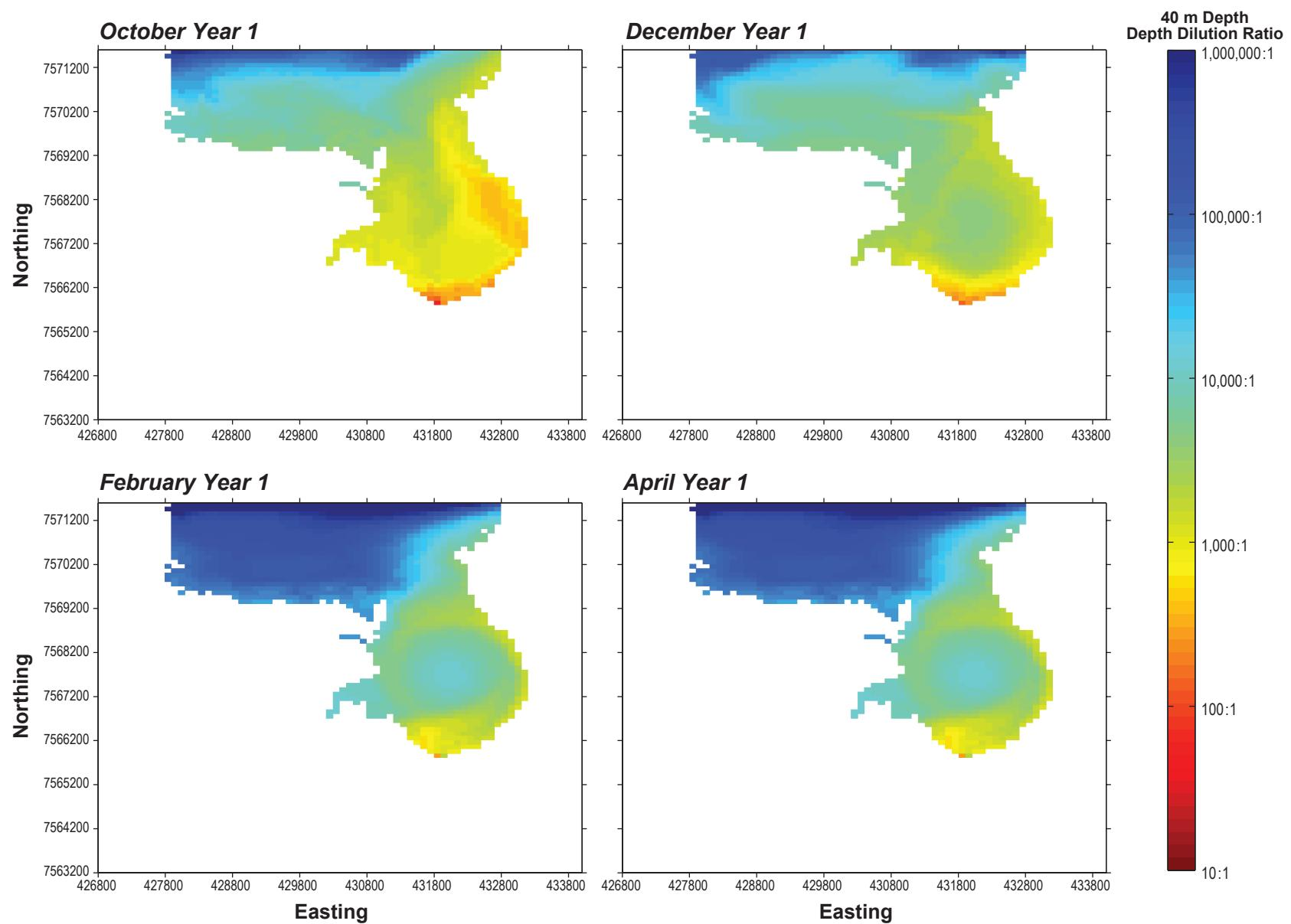
A total of three stations were included for monitoring timeseries of modelled chromium in Roberts Bay. The proposed discharge diffuser was located at 40 m depth in the southern portion of the bay and had varying flows and chromium concentrations due to Project activities. Baseline concentrations of chromium in Roberts Bay and from the other freshwater discharges were assumed constant to cleanly monitor the effluent plume propagation.
