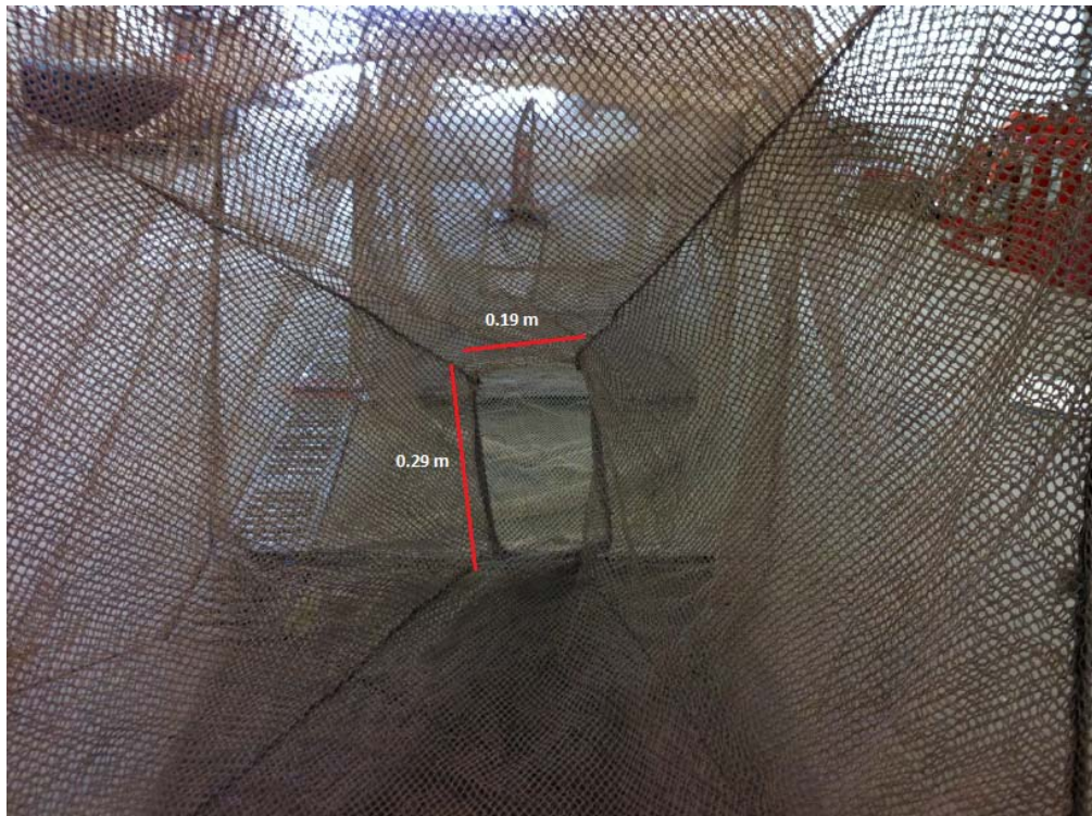
Photo 6: Fyke Net Internal Funnel Dimension
