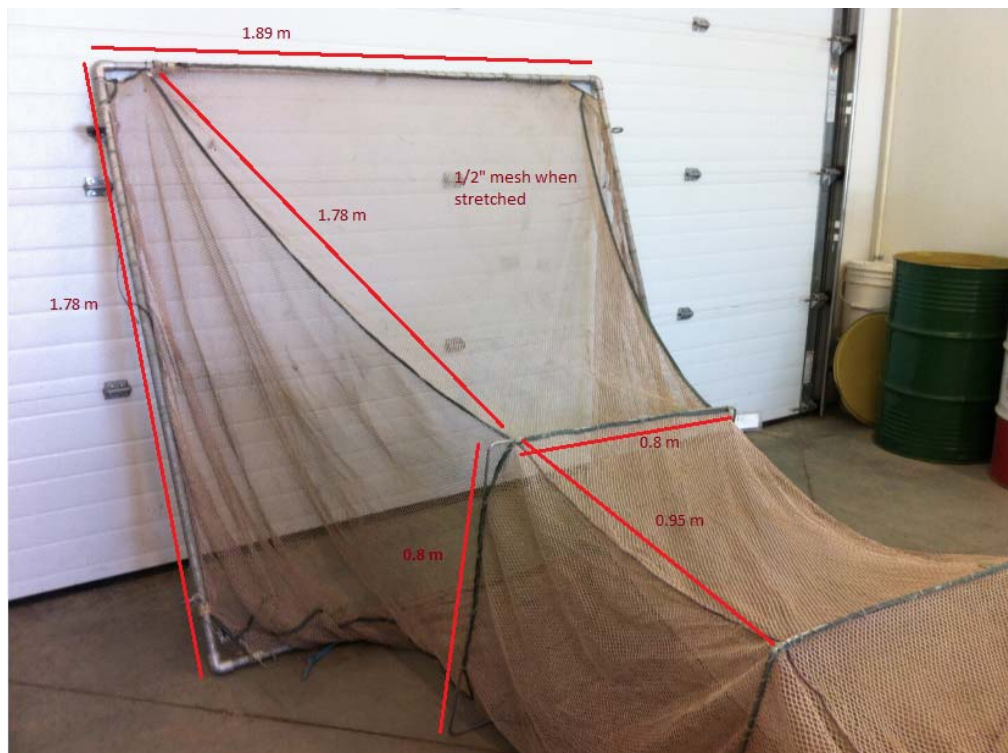
Photo 4: Fyke Net Throat Including Dimensions
