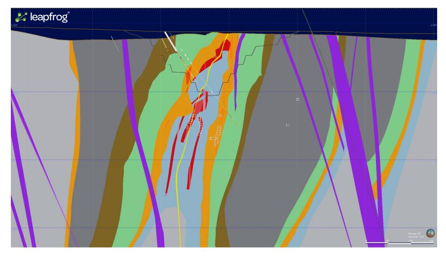
$Goose\ Main\ Cross\ Section\ 9:\ 550-600 m\ looking\ north-west.\ Drill\ collar\ 12GSE248C\ shown.$
