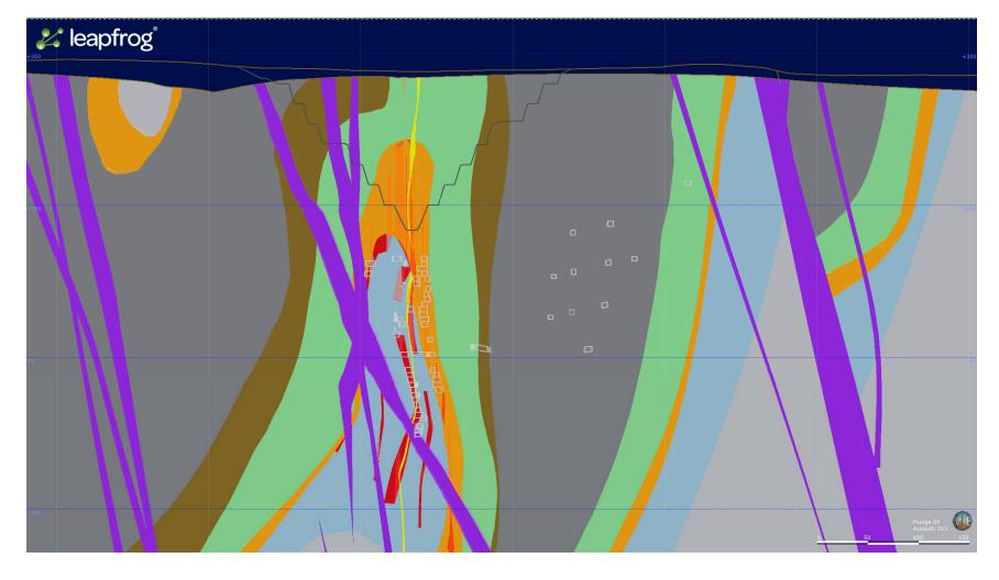
Goose Main Cross Section 6: 450 – 475m looking north-west. Drill collars 04GSE006, 00G0-03 and 00G0-25 shown from left to right. 12GSE245 enters cross section at top center from Goose Main Cross Section 5.
