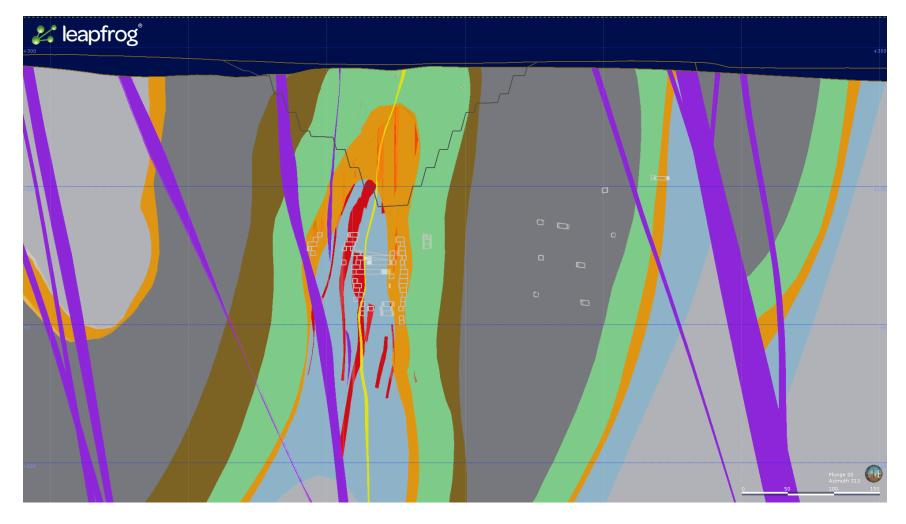
Goose Main Cross Section 7: 475 –500m looking north-west. Drill collars 00G0-02 and 04GSE022 shown from left to right. 13GSE286 enters cross section at top center from Goose Main Cross Section 8.
