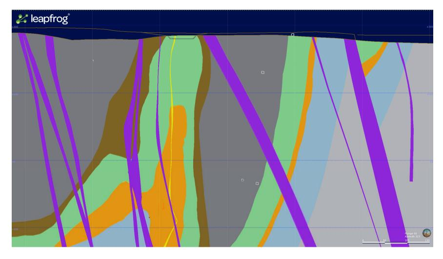
Goose Main Cross Section 4: 300 – 400m looking north-west. Drill collars SRK-11-GL-DH04, 08GSE008, SRK-11-GL-DH10 and 10GSE89 shown from left to right. 13GSE276 enters cross section at upper center from Goose Main Cross Section 3.
