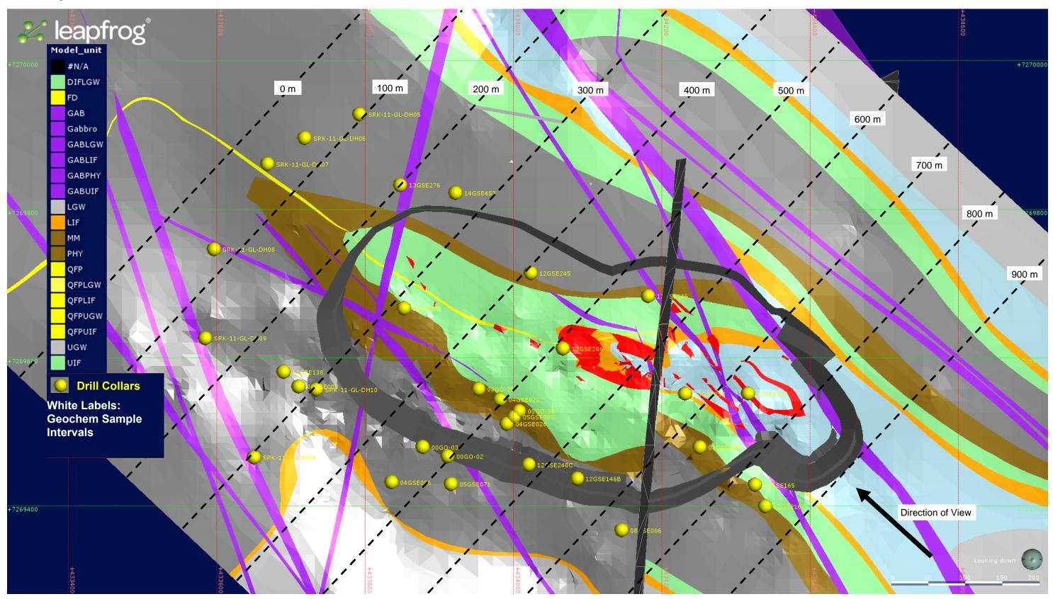
Goose Main Cross Section 1: 0 – 100m looking north-west. Drill collars SRK-11-GL-DH08, SRK-11-GL-DH07, SRK-11-GL-DH06, SRK-11-GL-DH05 shown from left to right. SRK-11-GL-DH09 enters cross section at lower left from Goose Main Cross Section 2.
