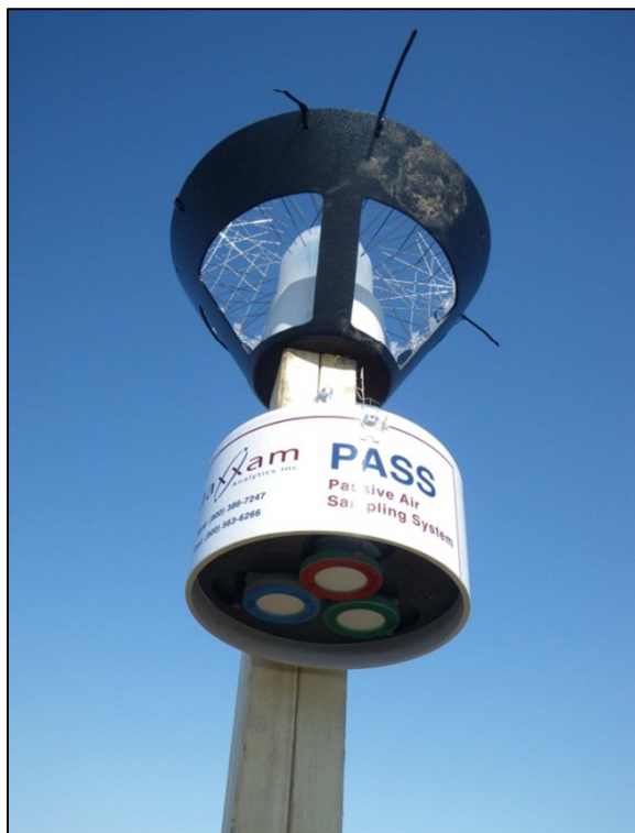
Plate 2.2-1. Close-up view of PASS sampler which measured \text{NO}_2 , \text{SO}_2 and \text{O}_3 .
