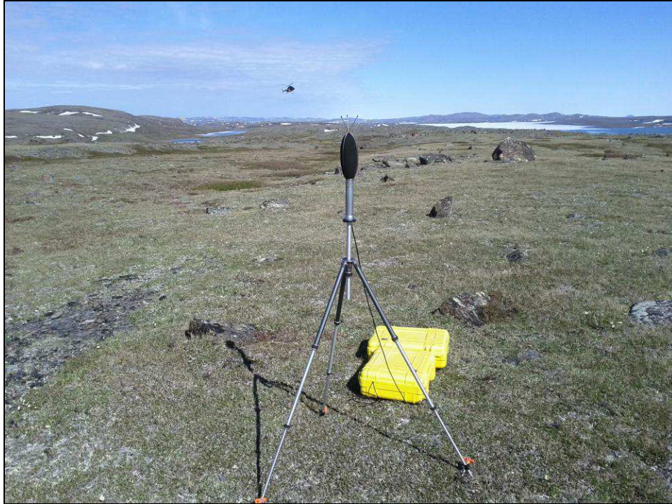
Plate 2-1. A typical sound level meter and associated environmental enclosure kits.
