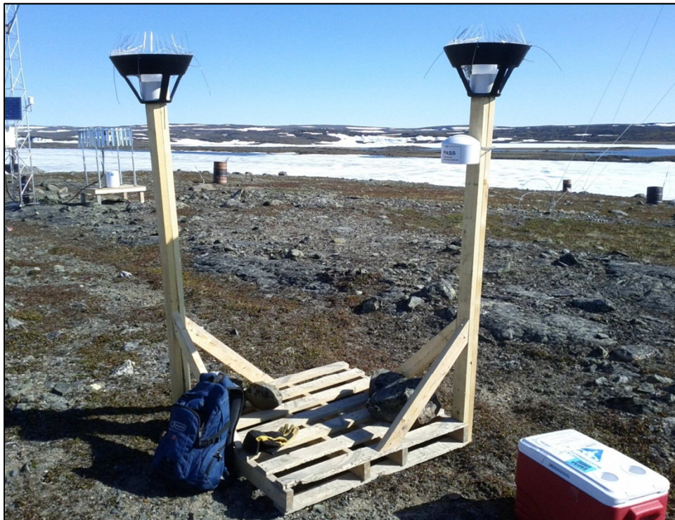
Plate 2.1-1. Dustfall station DF10 located within the George Property at the George Meteorological Station. The passive air sampling system shelter, for PASS2, can be seen on the right stand (June 17, 2012).
