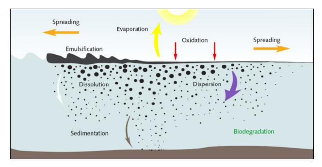
Figure 3.3-1. Schematic of Weathering Processes Acting on Spilled Diesel Fuel, Adapted from ITOPF (2011) and DHI (2012a)
