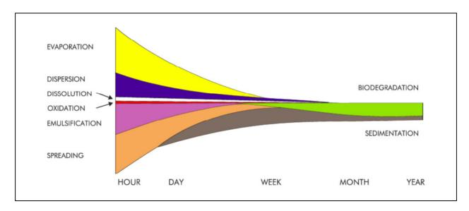
Figure 3.3-2. Heuristic Representation of the Relative Importance of Each Weathering Process on a Given Spill through Time - the Width of Each Band Indicates the Importance of the Process, Adapted from ITOPF (2011) and DHI (2012a)
