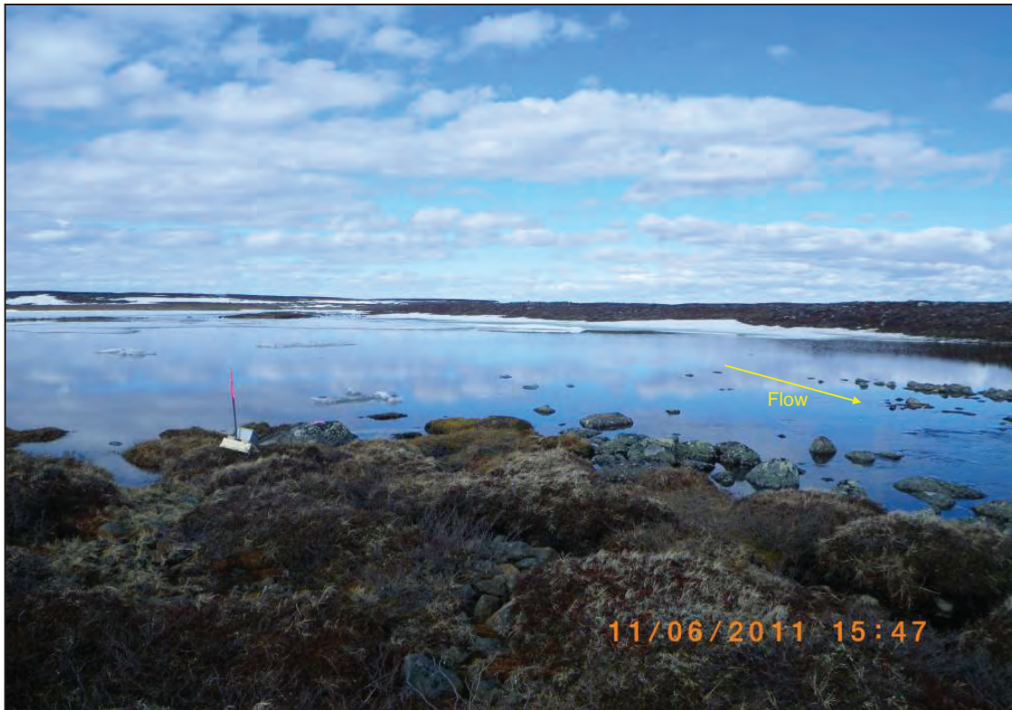
GI-H1, looking out over Giraffe Lake where the station is located at the outflow. The stage at the transducer location is governed by a section control located downstream in the channel. The section control is a riffle where boulders protrude from the water surface at all stages. Photograph taken on June 11, 2011.
