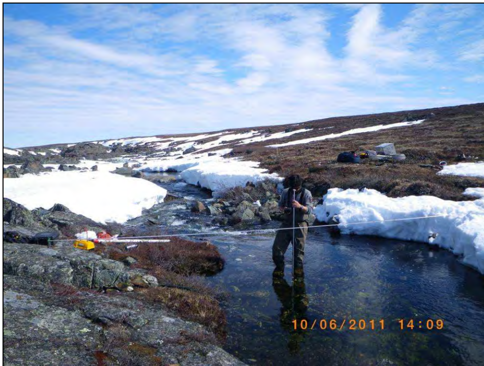
Plate 3.3-1. Velocity-area discharge measurements at hydrometric station GL-H1 using a handheld current velocity meter. Photograph taken on June 10, 2011.
