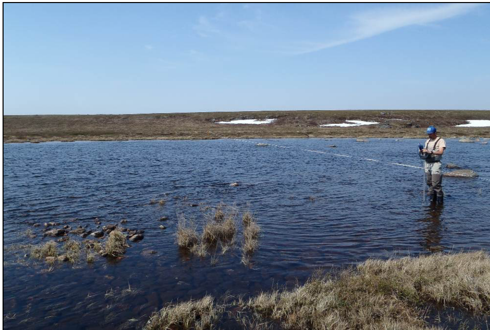
Plate 3.4-2. Velocity-area discharge measurements at hydrometric station PL-H2 (Propeller Lake Inflow) using a handheld current velocity meter, June 18, 2014.
