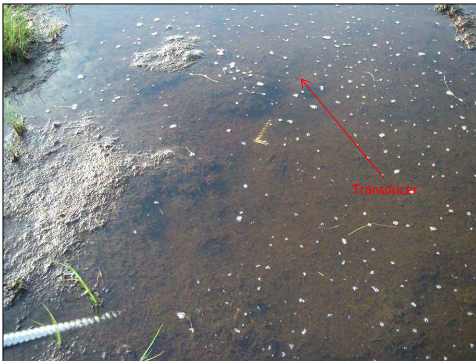
Plate 4.2-1. Close up view showing the transducer submerged in the thawed stream bed late in the summer at the hydrometric monitoring station REFB-H1. Data recorded in the levelling surveys conducted over the field season were used to correct for the change in elevation of the transducer. Photograph taken on August 15, 2011.
