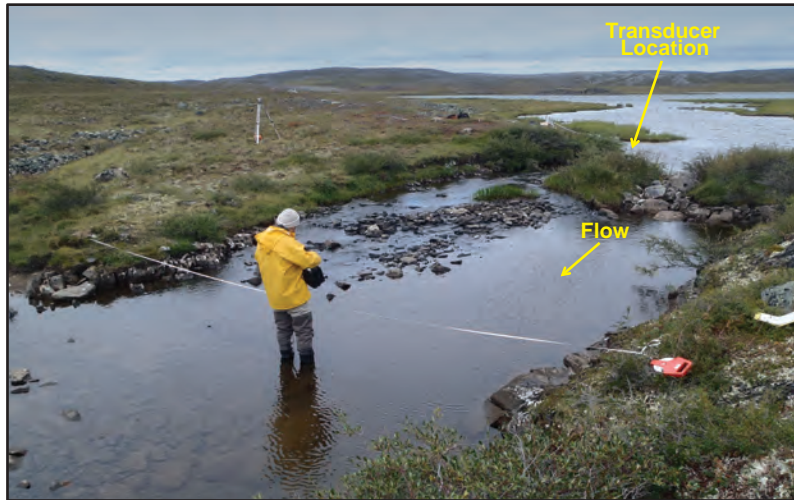
Upstream view of station KL-H2 on George Lake outflow during a flow measurement. The pressure transducer is located in George Lake with the flow gauging section downstream of the outlet. Photograph taken August 12, 2012.
