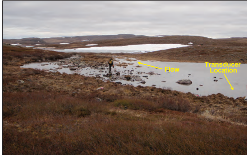
REFC-H1, looking downstream towards the monitored reach. The channel is characterized by vegetation and rocks with the flow splitting in two sections along its length. The pressure transducer is located in Reference Lake C near the outlet. Photograph taken June 11, 2012.
