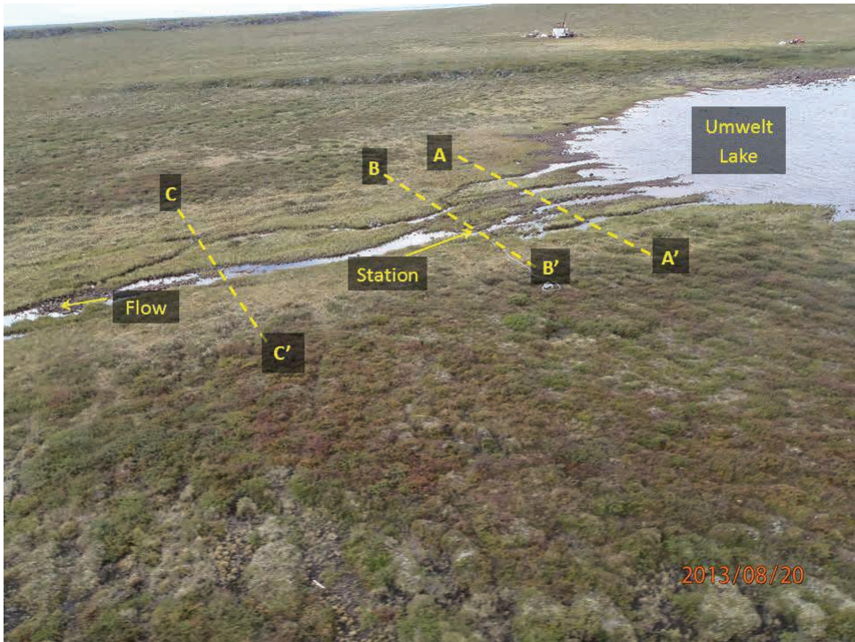
Aerial view of station UM-H1 and the surveyed channel reach – cross-sections A (12 m upstream of station), B (at station), and C (18 m downstream of station). August 20, 2013.
