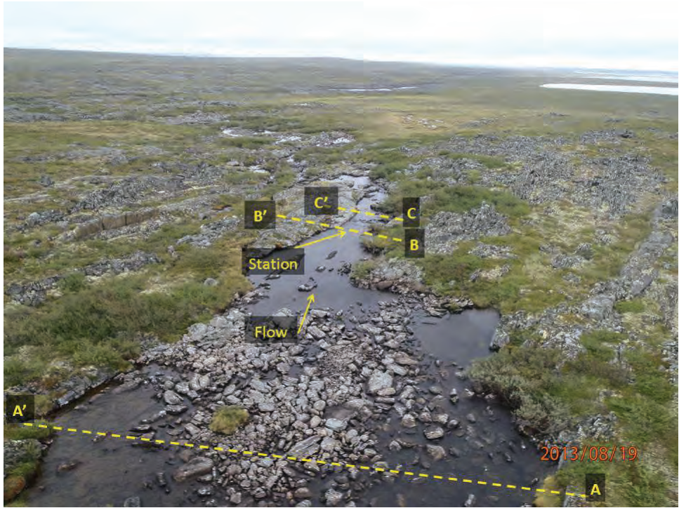
Aerial view of station WP-H1 and the surveyed channel reach – cross-sections A (20 m upstream of station), B (at station), and C (5 m downstream of station). August 19, 2013.
