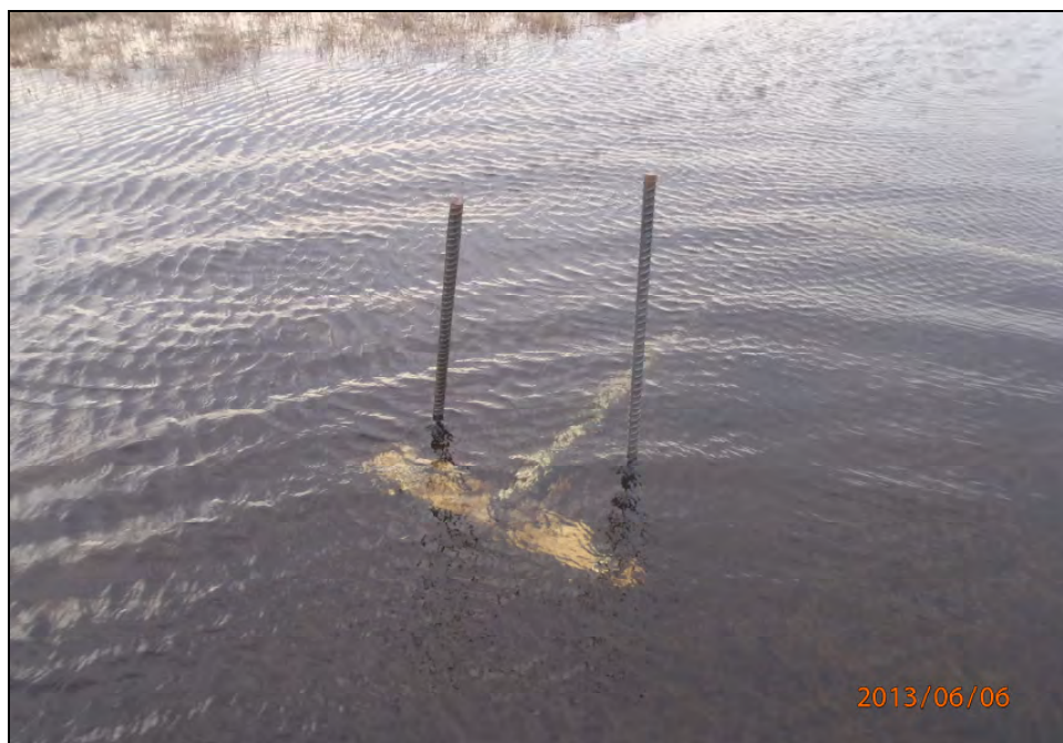
Plate 4.2-1. Station set-up at REFB-H1 in 2013. Rebar was used in an attempt to limit vertical drift of the transducer into the soft bed along the channel reach. June 6, 2013.
