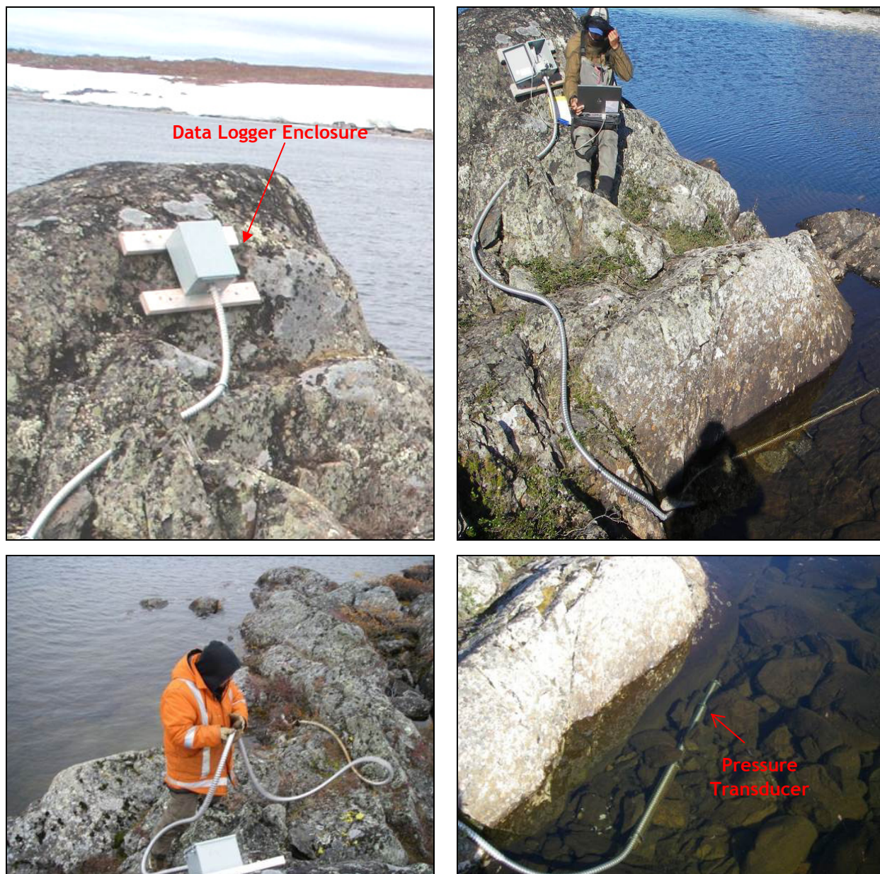
Plate 3.2-1. Photographs illustrating the hydrometric monitoring station design.
