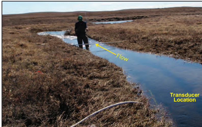
BL-H3, looking downstream along the monitored reach with the transducer location in the foreground. The rod across the channel indicates where manual flow measurements were conducted. Photograph taken June 12, 2012
