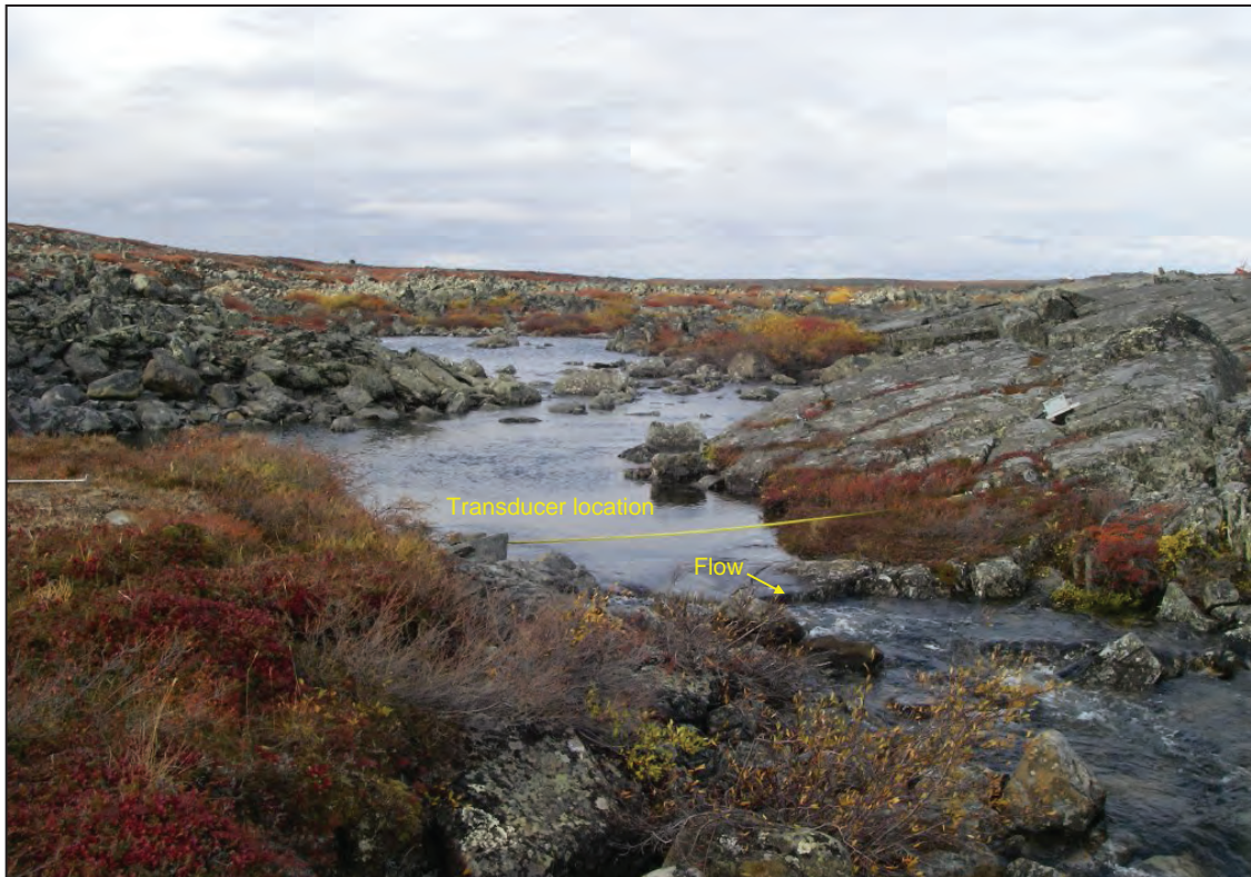
GL-H1, looking upstream along the monitored reach. The water elevation in the pool where the transducer is positioned is controlled by the bedrock channel constriction downstream. The yellow tape across the channel indicates the channel cross section where manual flow measurements were conducted. Photograph taken September 16, 2011.
