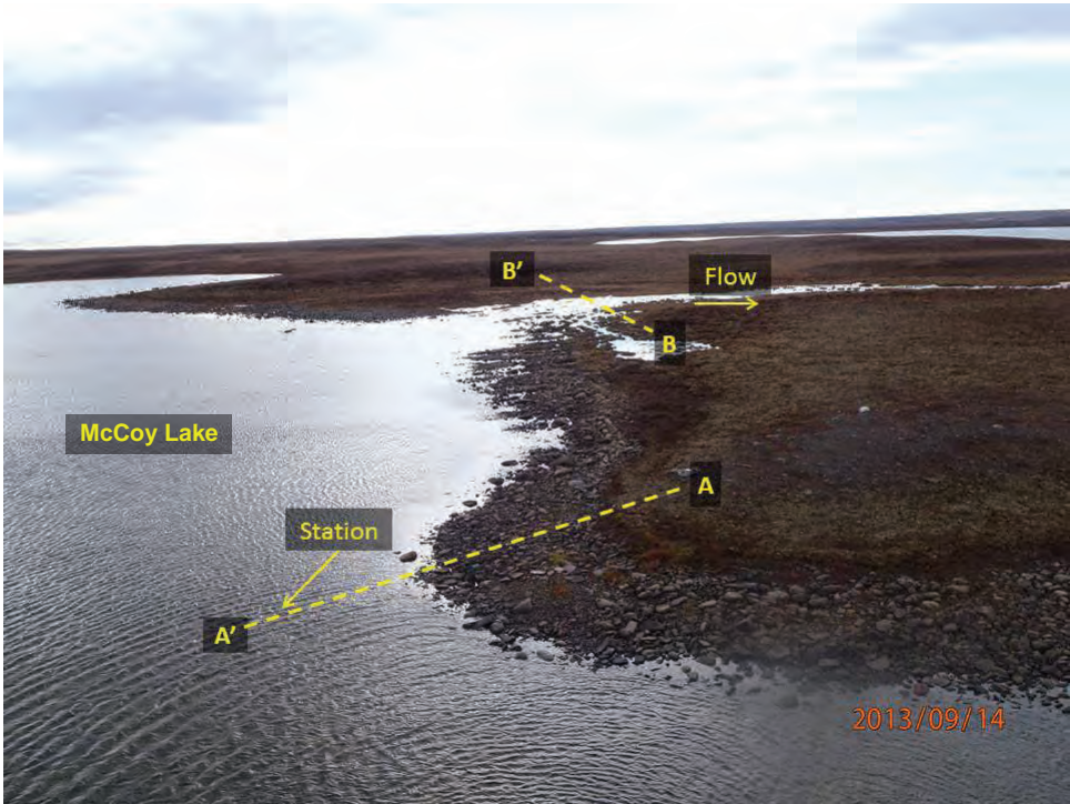
Aerial view of station Mc-H1 and the surveyed channel reach – cross-sections A (shoreline profile at station) and B (lake outlet 150 m downstream of station). September 14, 2013.
