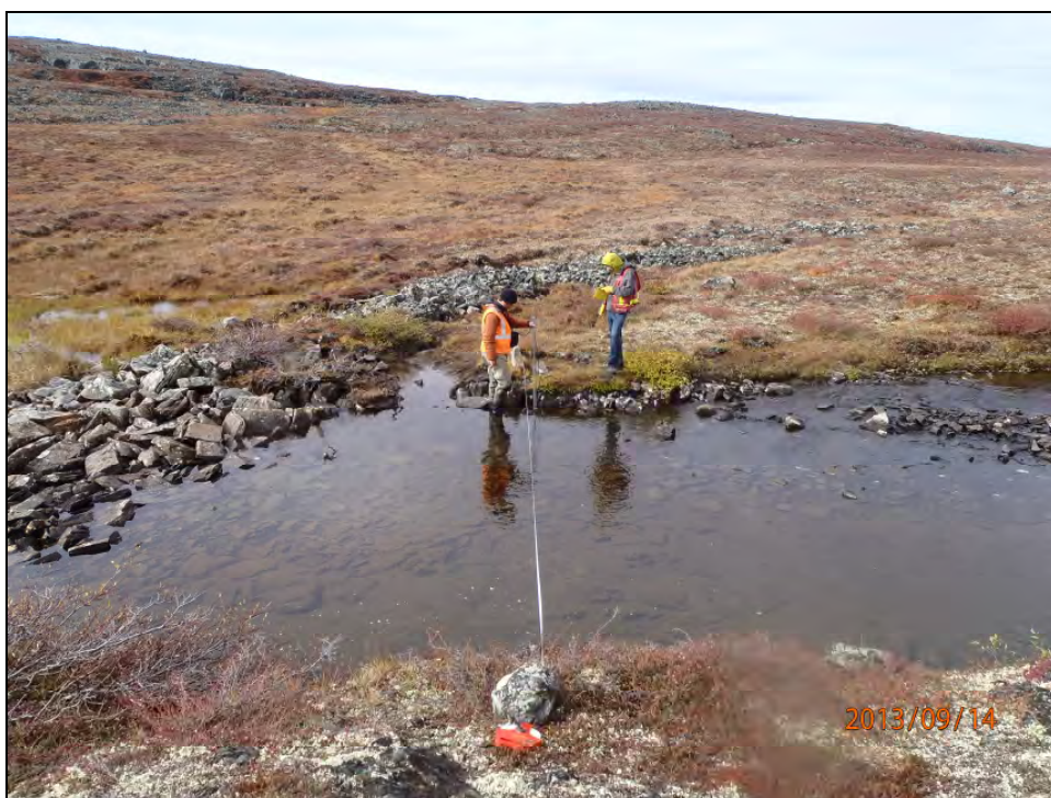
Plate 3.3-1. Velocity-area discharge measurements at hydrometric station KL-H2 using a handheld current velocity meter. September 14, 2013.
