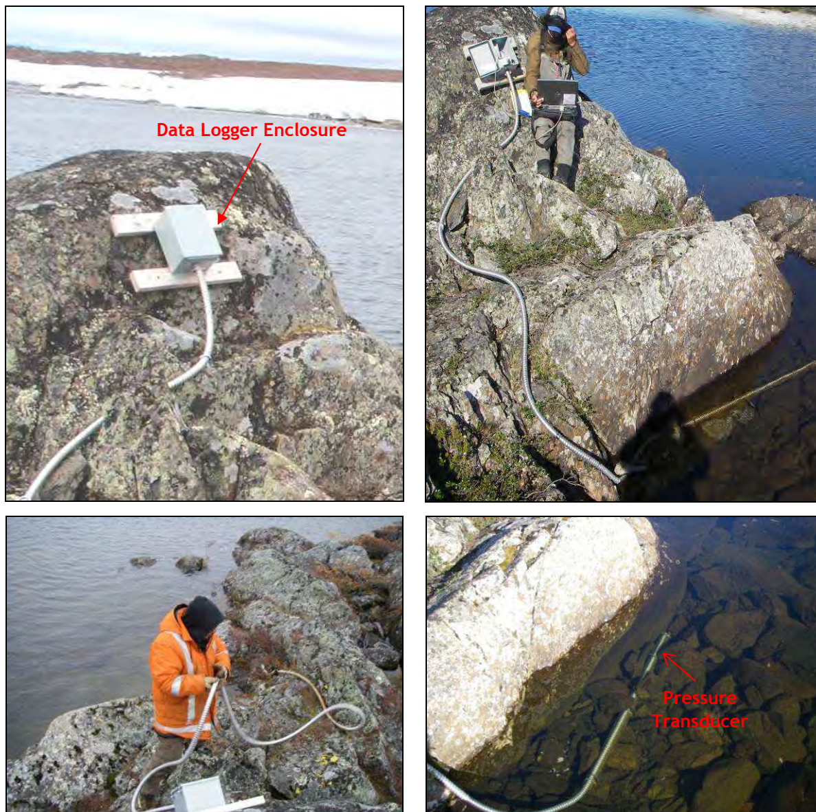
Plate 3.2-1. Photographs illustrating the hydrometric monitoring station design.
