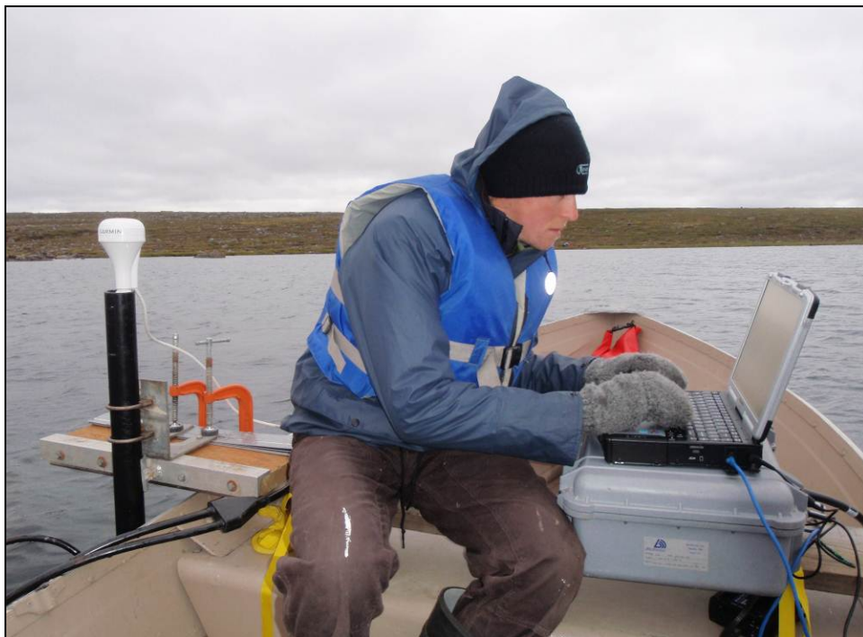
Plate 2.1-2. BioSonics hydroacoustics system used to classify substrate and estimate fish populations, Umwelt Lake, Back River Project, 2010.
