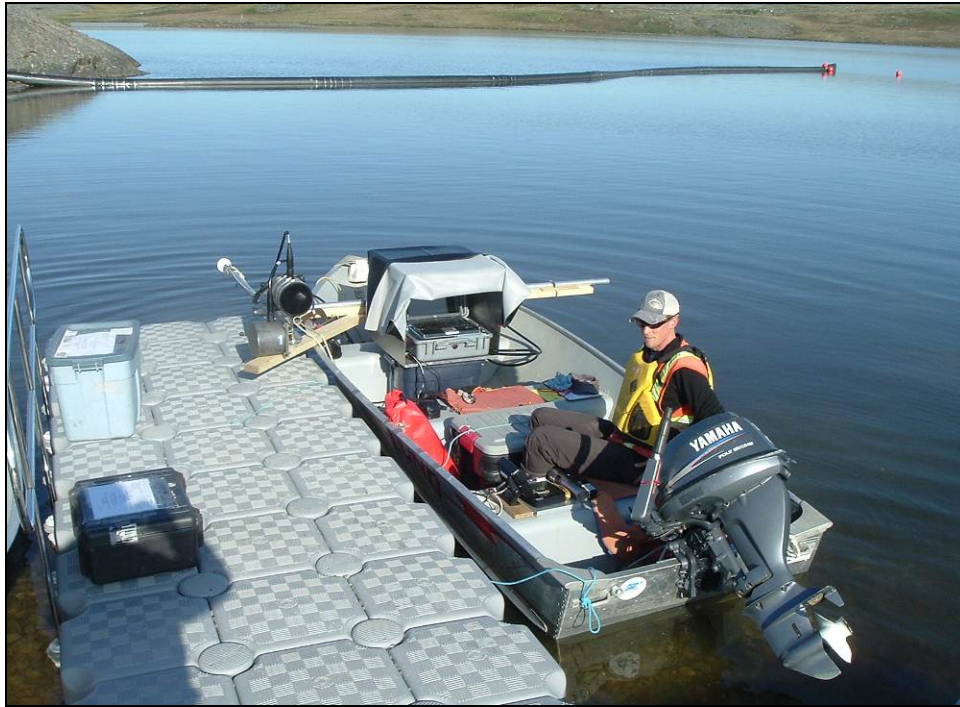
Plate 2.1-1. Boat set-up used to conduct hydroacoustics surveys of Llama and Umwelt lakes, Back River Project, 2010.
