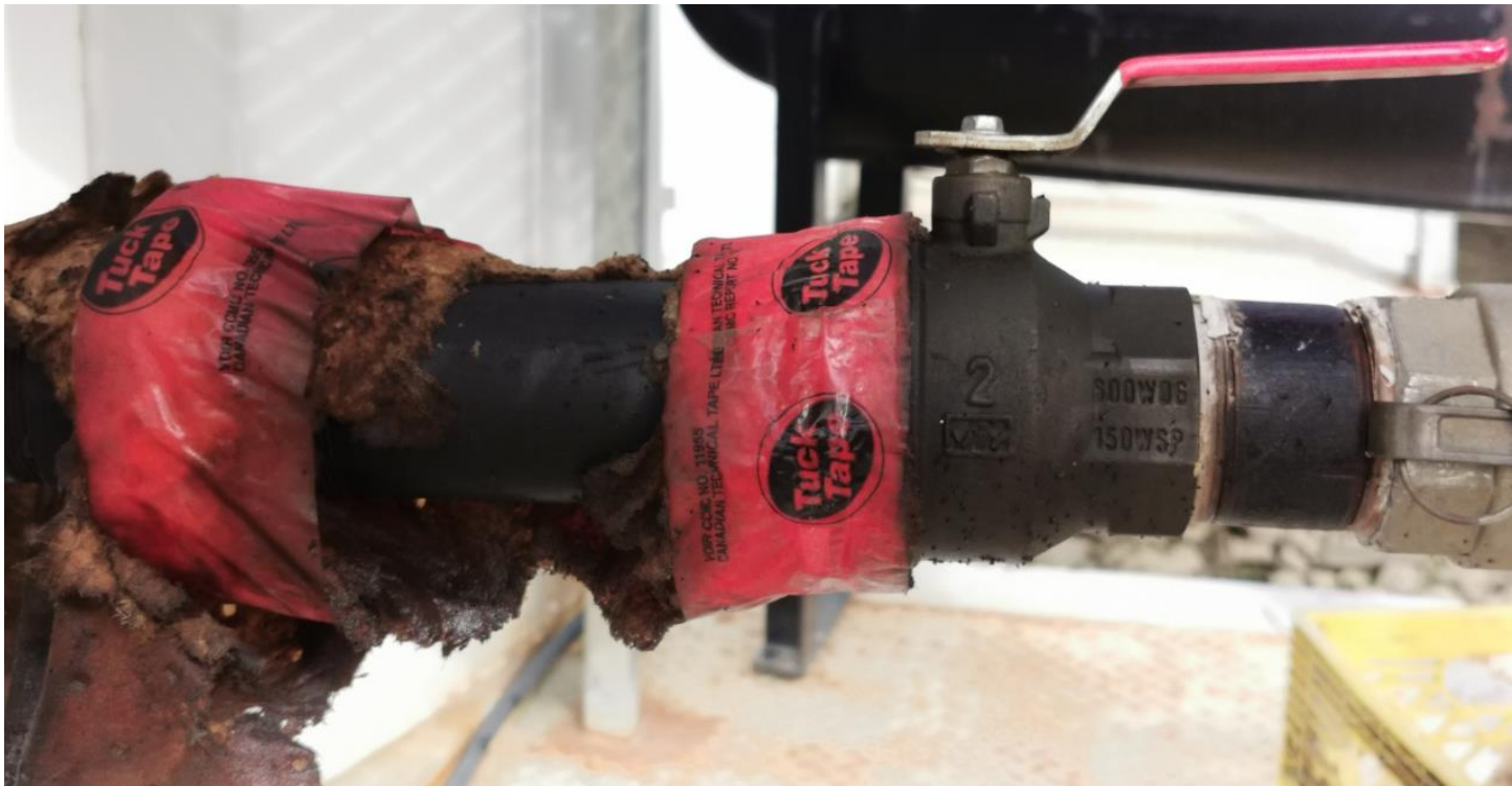
Coupling device attached to tank number 7 where the spill occurred from. Improper temporary fix in order to prevent further discharge.
