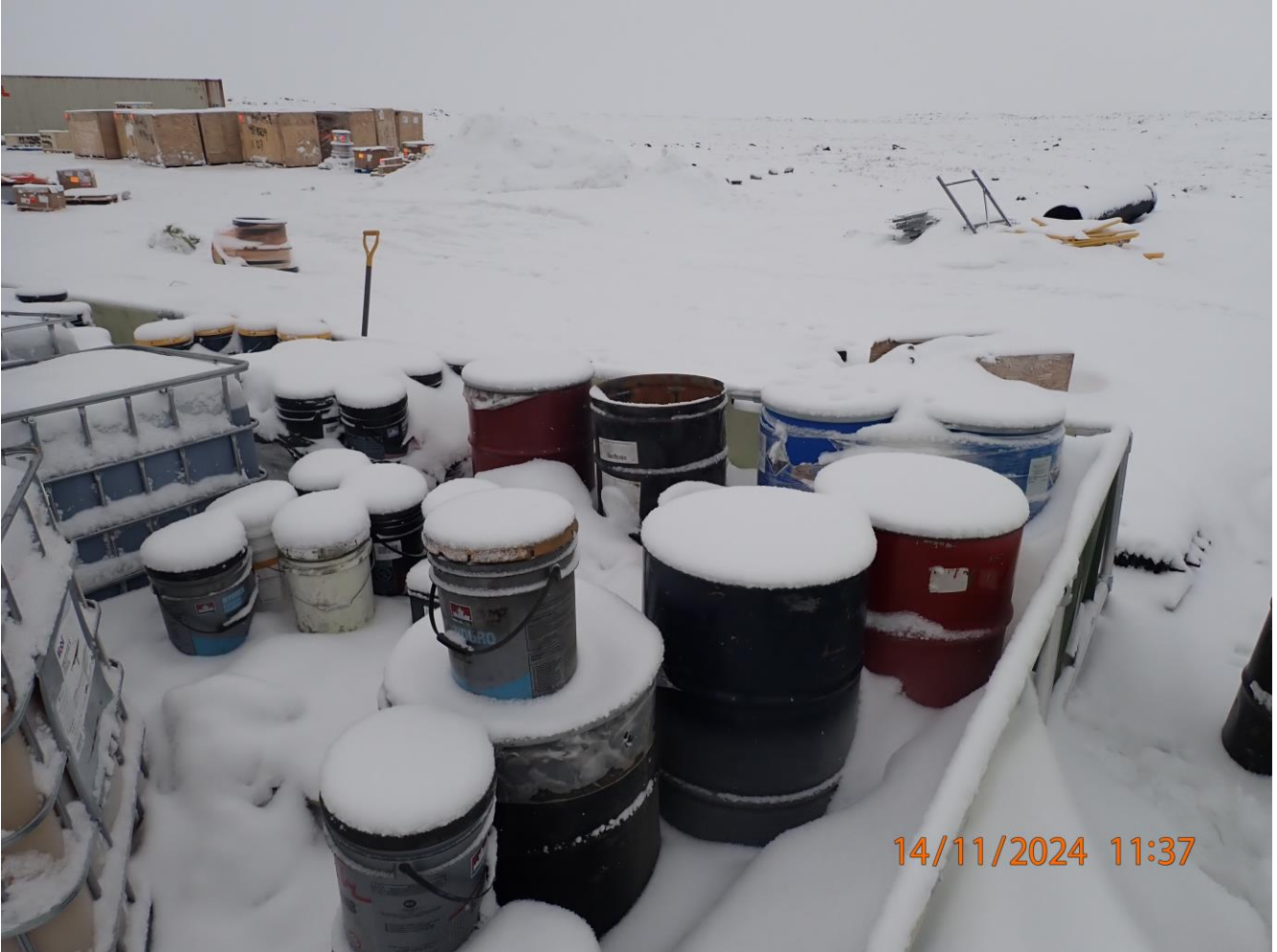
Open container inside insta berm. Hazardous waste containers shall be sealed from the elements.
