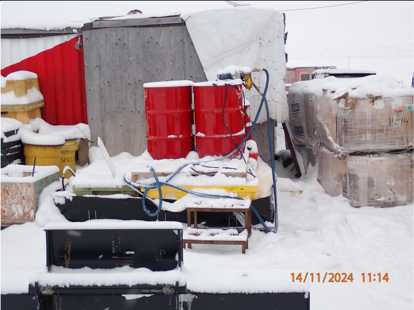
Fuel drums stored in secondary containment, refuelling hose not in containment.
