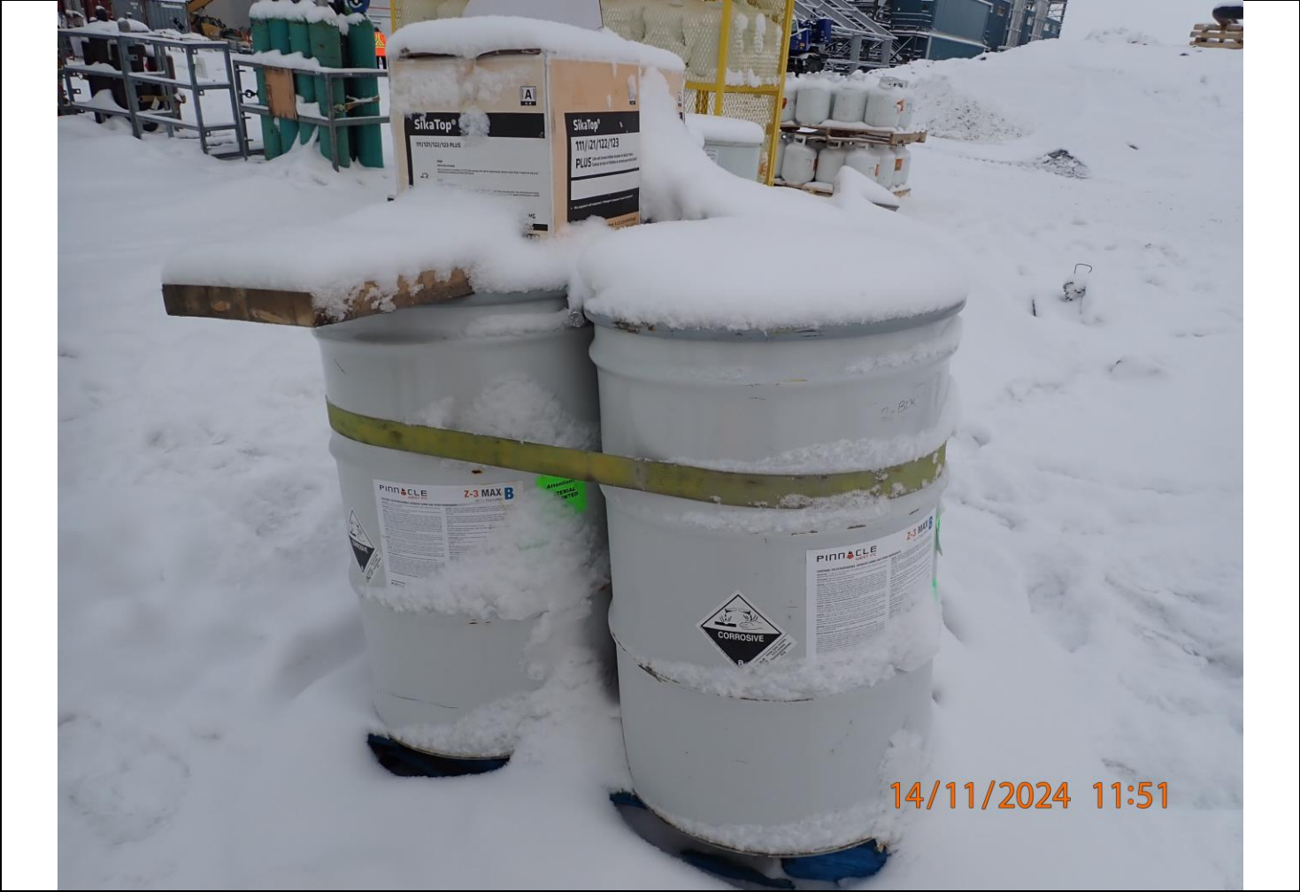
Z-3MAX stored outside of secondary containment, corrosive material sticker shown.
