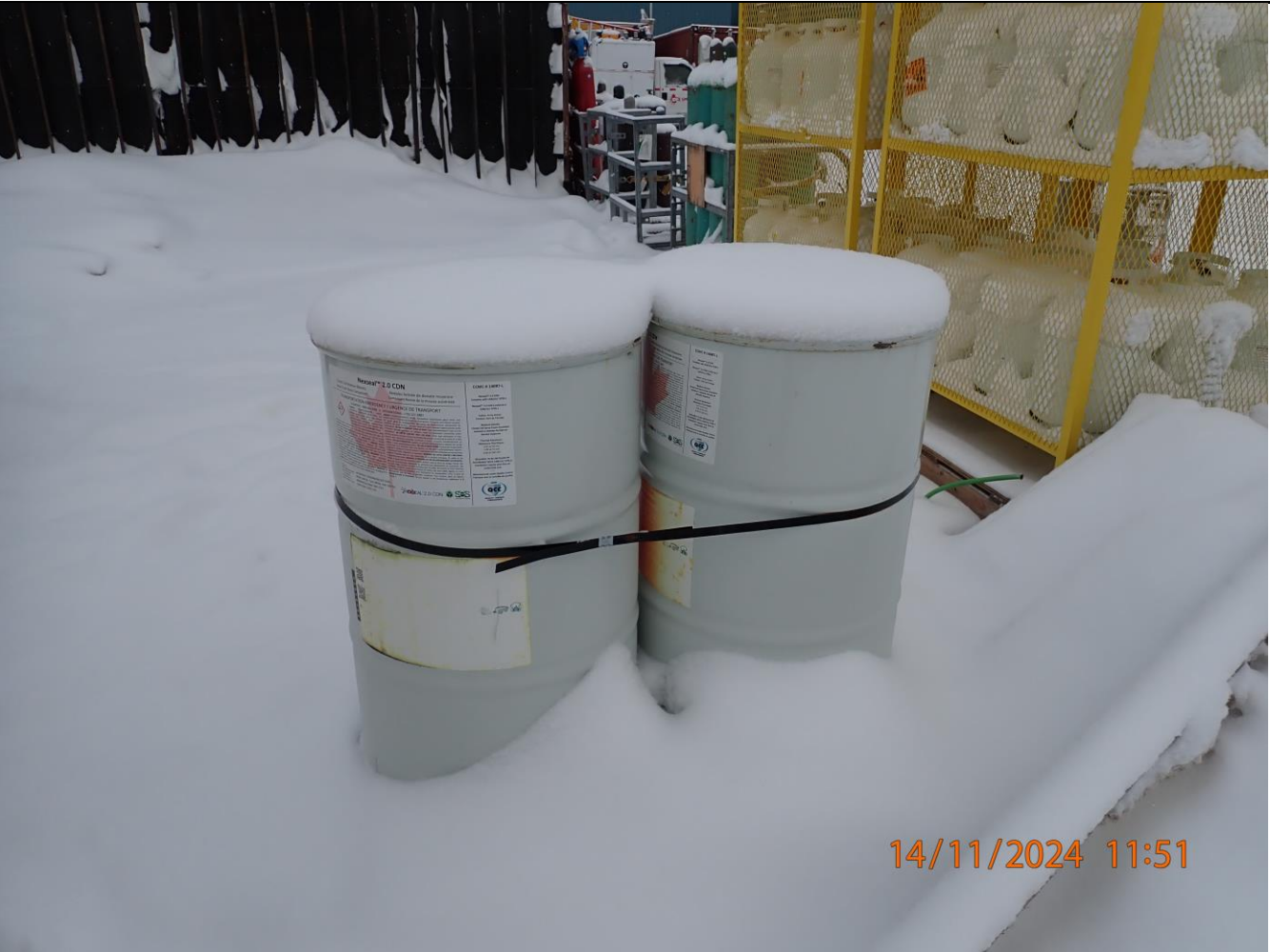
Nexseal 2.0 stored outside of secondary containment
