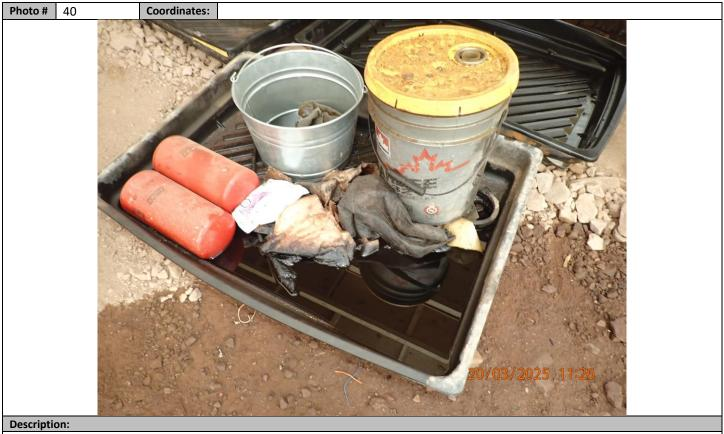
Oil drip tray filled with oil, oil filters, buckets and oily rags.
