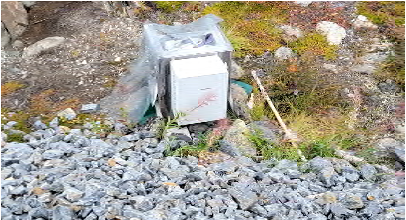
G-88. – Ground temperature monitoring station at the western toe of the Neck Crossing road
