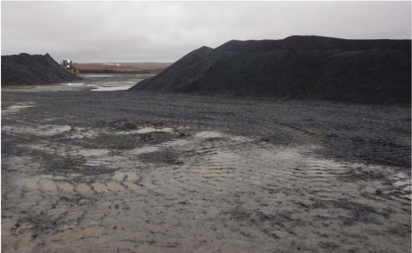
G-26. - Crusher stockpile pad. Two piles of 1” crush
