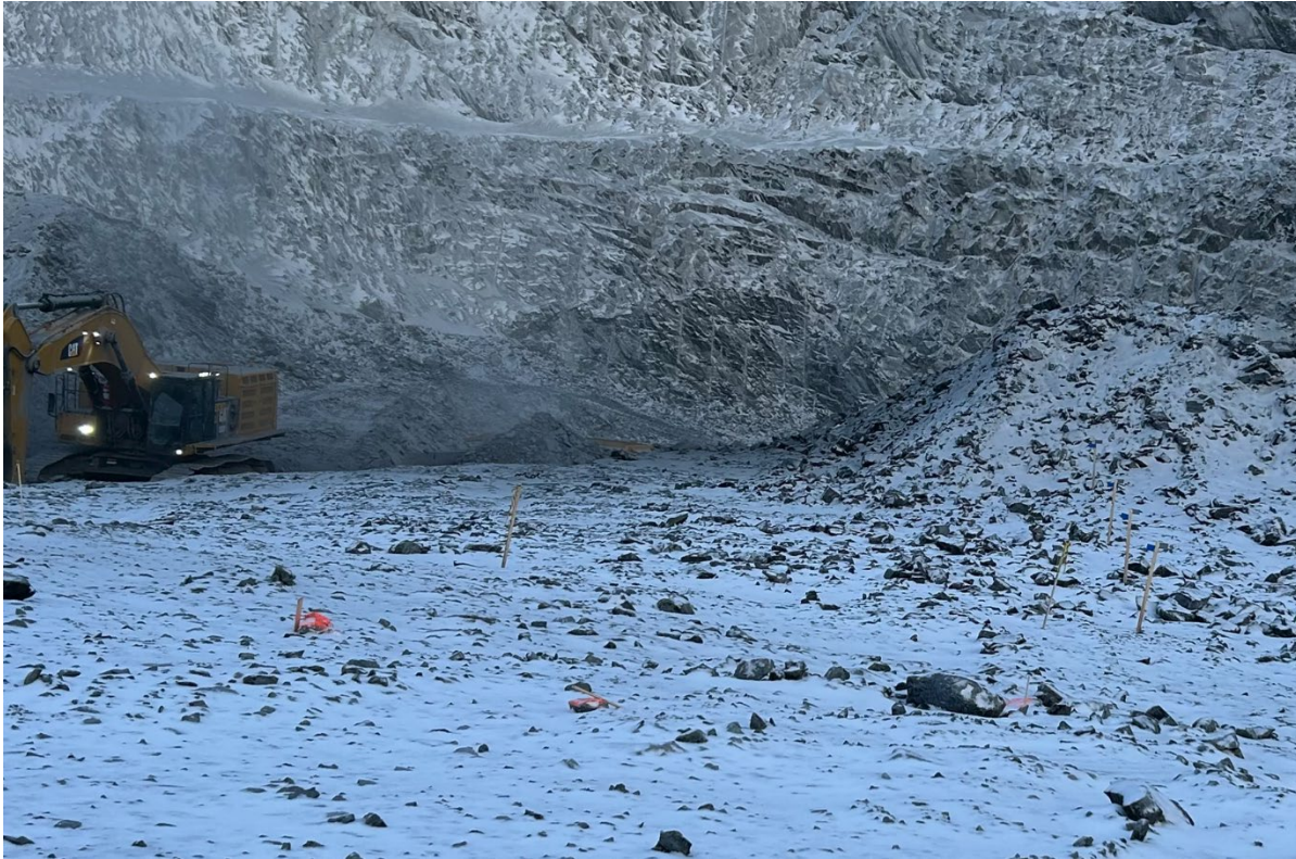
Figure 2: Survey markers (right side of picture) designating NPAG and PAG dig lines
