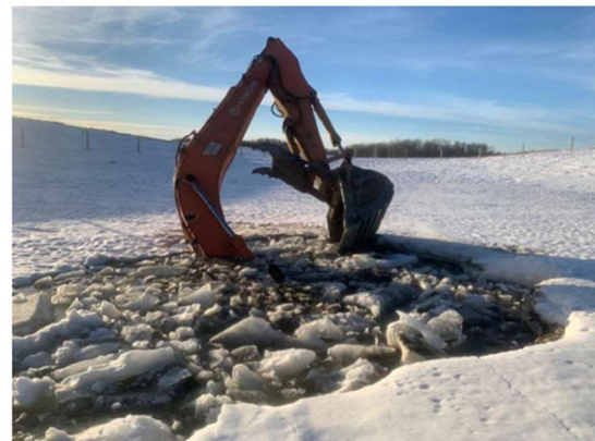
Figure 6 Excavator breakthrough on an ice cover over a dugout (Alberta OHS, 2023)
