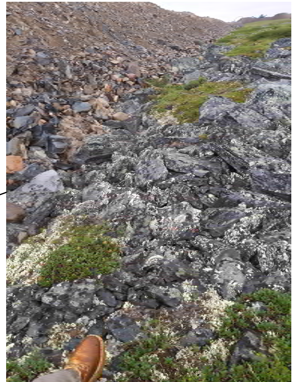
Photo 16 – Fractured rock extending under CWO embankment area
