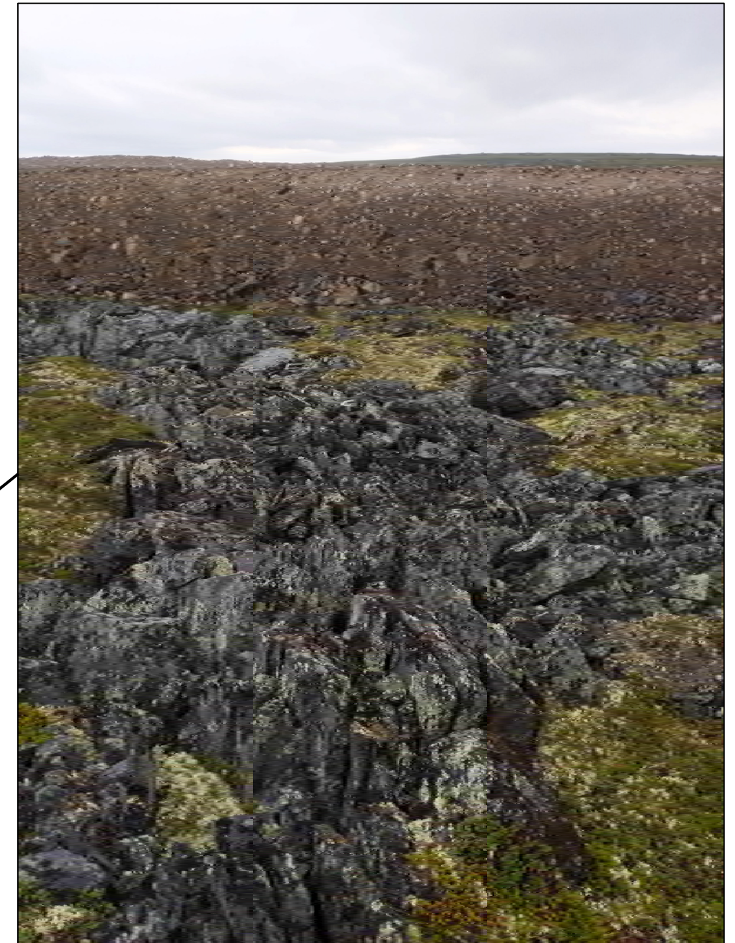
Photo 27 – Highly fractured rock outcrop extending through planned embankment area
