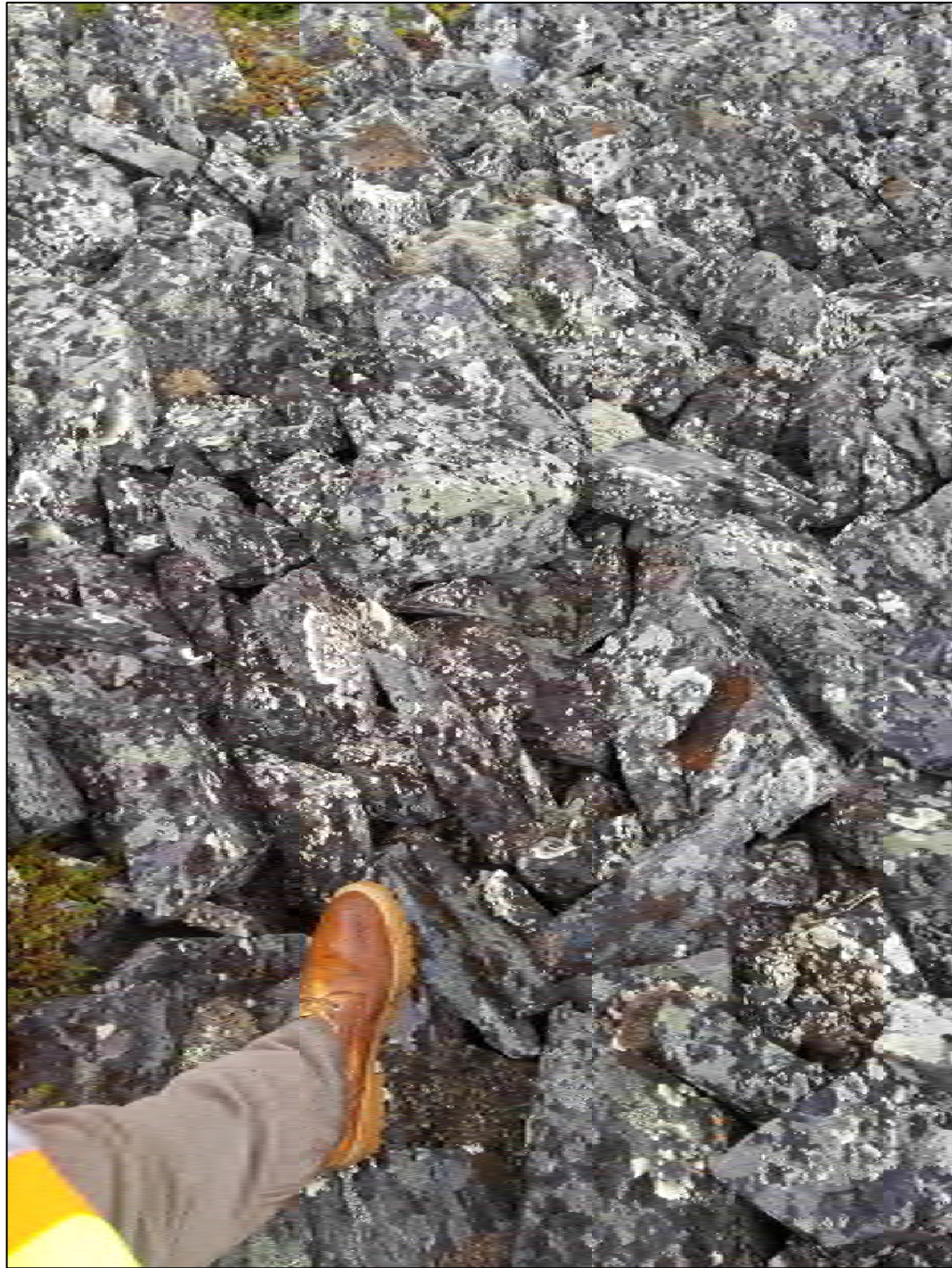
Photo 26 – Highly fracture rock outcrop
