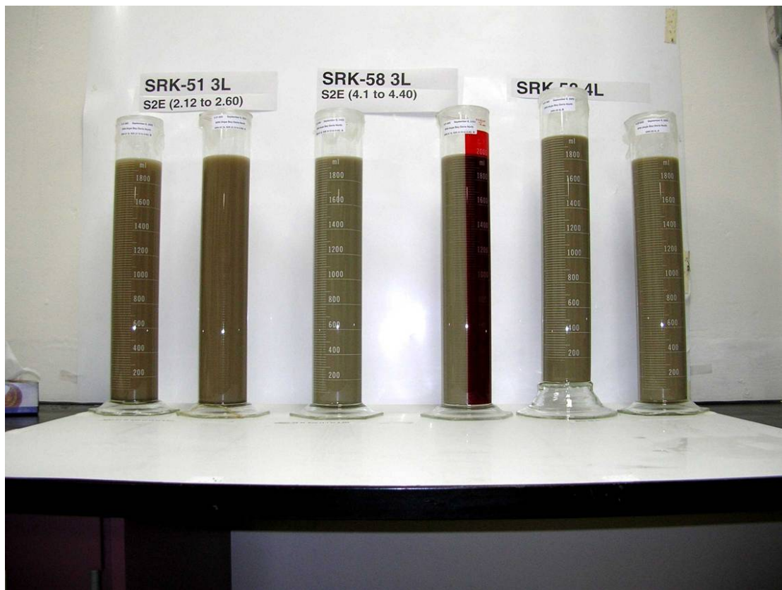
Photo 1. Settling Tests at Time = 0 hr
