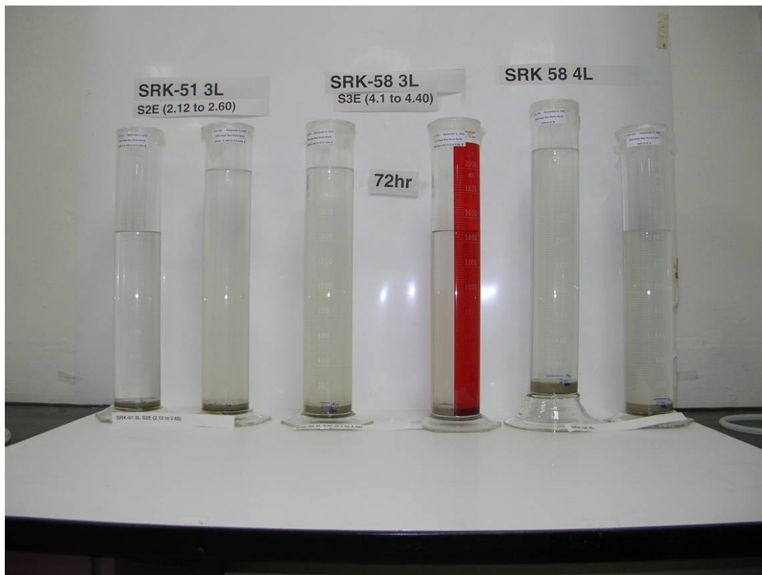
Photo 7 Settling Tests at Time = 72hr
