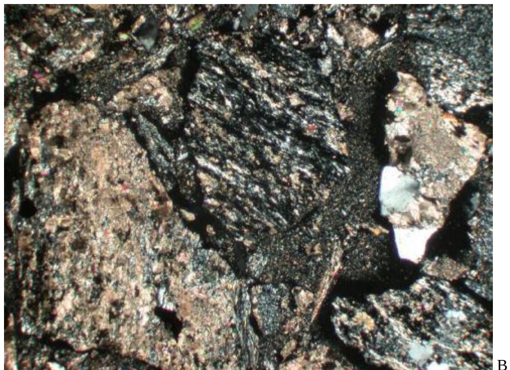
HC-32: A&B) View of banded quartz-chlorite-rutile-sericite-carbonate aggregate with disseminated opaques (pyrite) and quartz-carbonate vein fragment (right). A) PPL, B) XPL, FOV \approx 4.5 mm.
