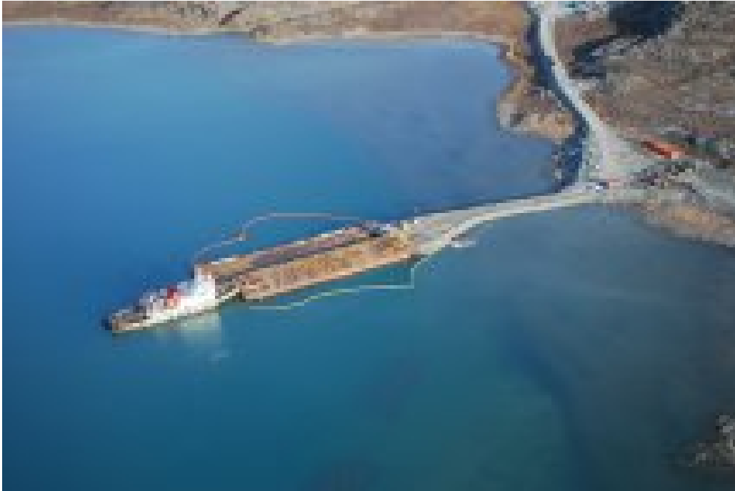
Photos show Oil Containment Boom surrounding Fuel Barges
