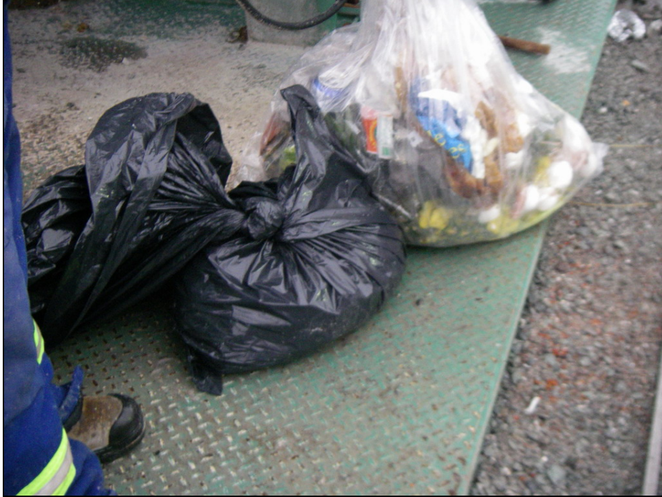
Plate 2.1-4. Two bags of camp waste were introduced into the Doris incinerator every 90 to 110 minutes during the September/October 2009 stack emissions testing campaign. The black bag contains “dry” waste (i.e., biosolids) from the on-site sewage treatment plant and the clear bag contains “wet” kitchen waste.
