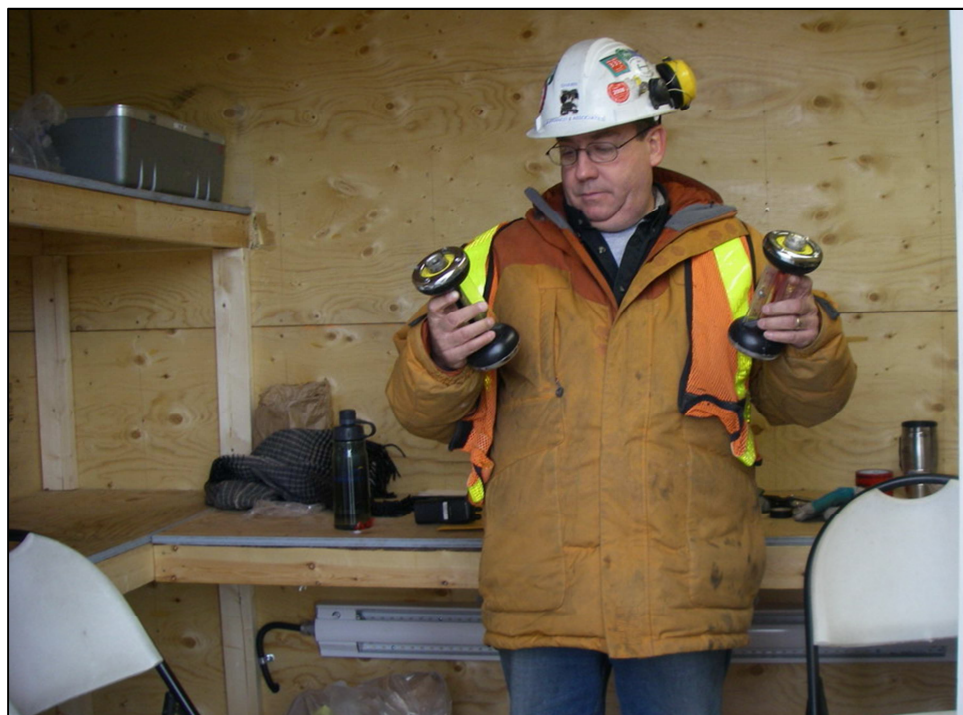
Plate 3.1-1. The O 2 and CO 2 concentration in the stack gas was determined using portable Fyrites analyzers.
