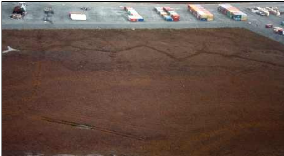
Photo 12: Rimpull Rolygon tracks on a tundra test plot near all-weather road
