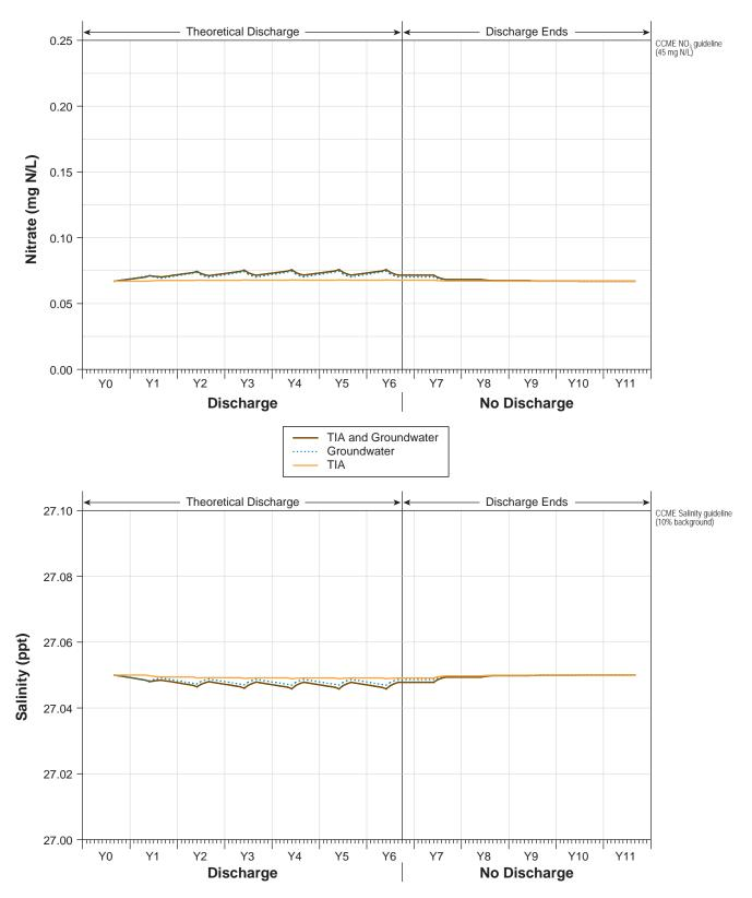
Note: Allowable effluent concentrations are based on continuous 80 L/s of TIA and groundwater discharge during the open-water season, 45 L/s of TIA discharge during the open-water season, and 35 L/s of groundwater discharged over the year.
