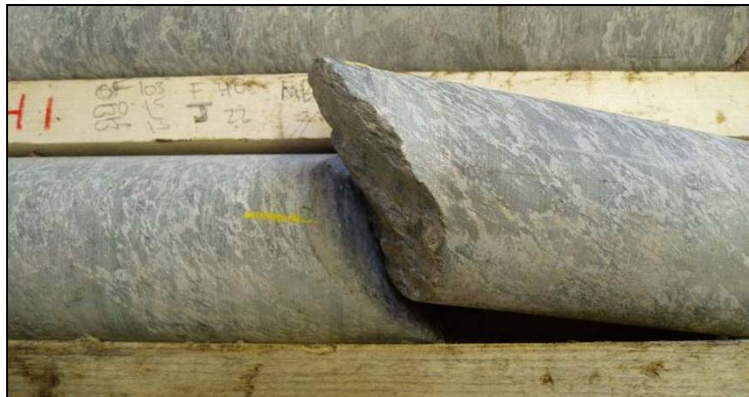
Although sub-parallel to foliation, roughness and angularity of break indicate mechanical damage.
