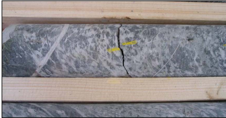
Note high angle, very fresh break indicating drill damage.
