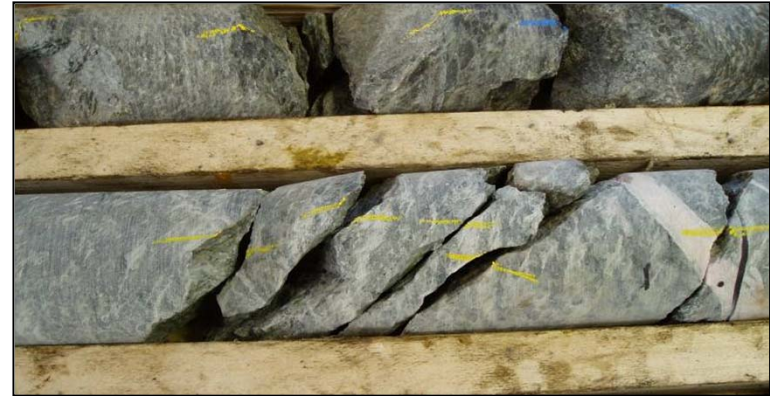
Cluster of foliation sub-parallel fractures – roughness and angularity indicate mechanical damage.
