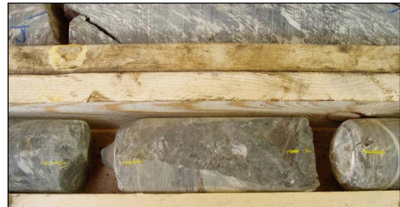
"Drill spin" is an obvious indication of mechanical damage.
