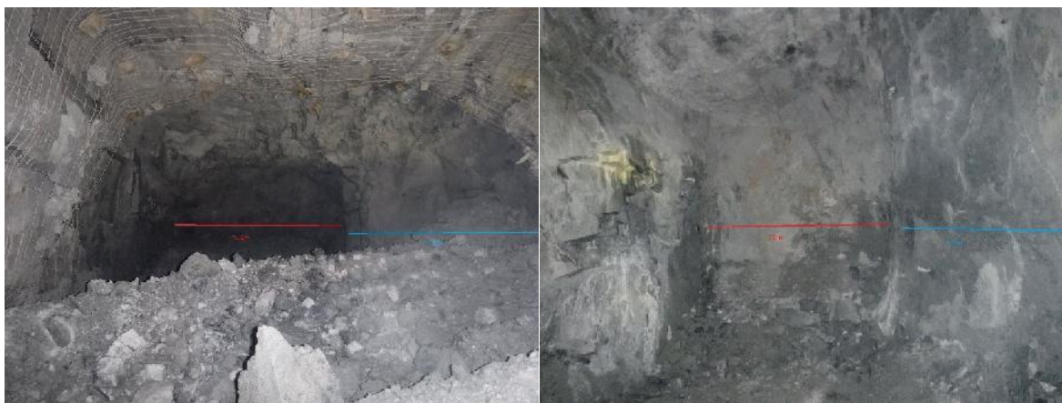
Figure 5: After cast blasting and after mucking a resued round (4966 level) to improve grade, left (red) is ore and right (cyan) is waste.
