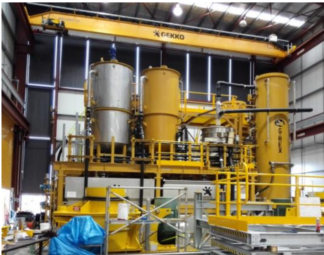
Figure 10: Resin column module in factory acceptance testing at Gekko's Ballarat facility.
