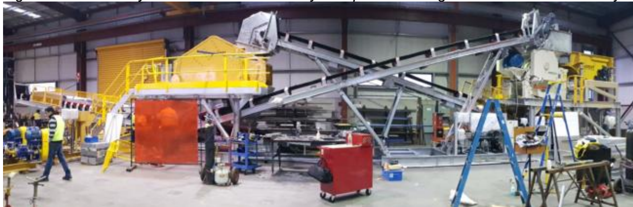
Figure 11: Secondary crusher module in factory acceptance testing at Gekko's Ballarat facility.
