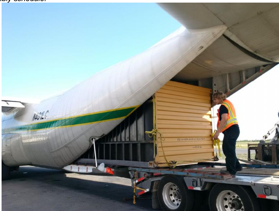
Figure 12: Loading MCC modules for delivery by C130 Hercules aircraft to Hope Bay on specially designed skids. The MCC's were the largest volume item capable of being transported on this type of aircraft. The 10 MCC modules were airlifted to site to accelerate the Processing Plant assembly schedule.
