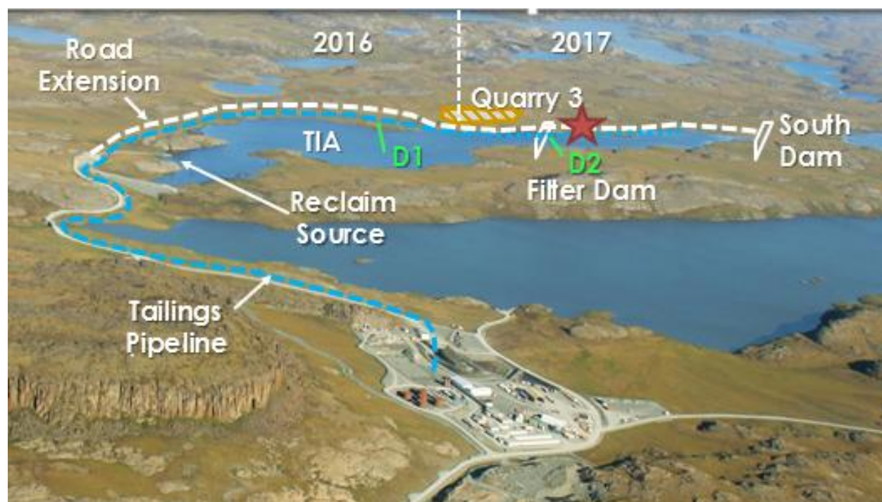
Figure 8: TIA road development progress. The star indicates location at June 30, 2016 and the vertical line just left of Quarry 3 was the extent of the planned 2016 scope of work. D2 is the location of initial subaerial tailings disposal
