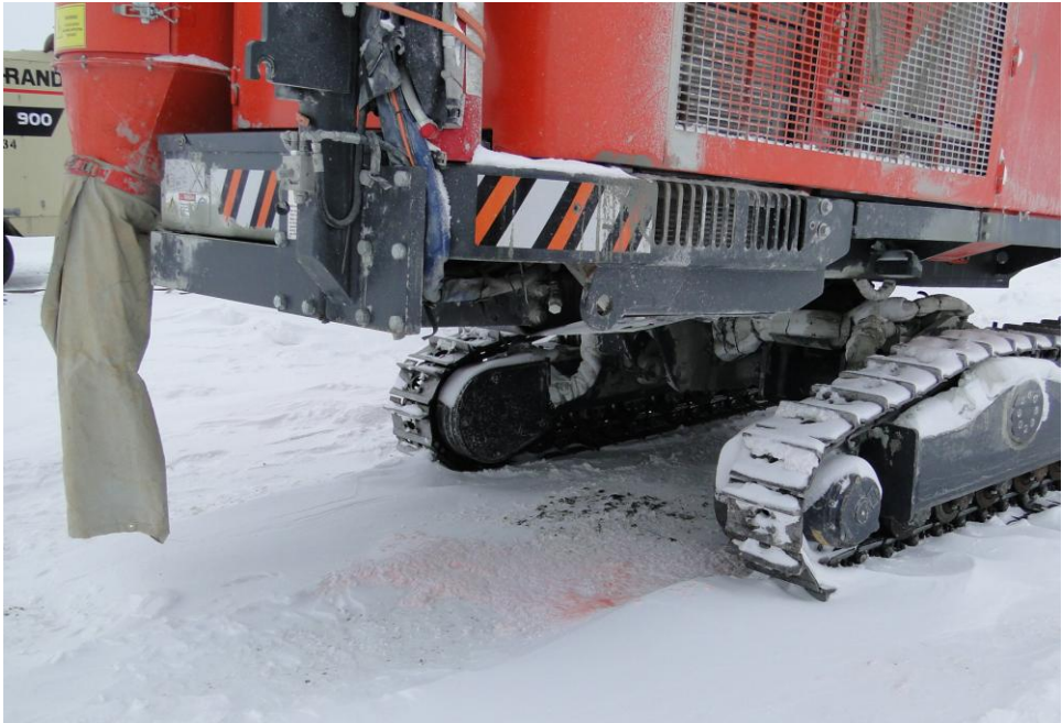
No drip tray or absorbent under drill outside McCaw North shop.
