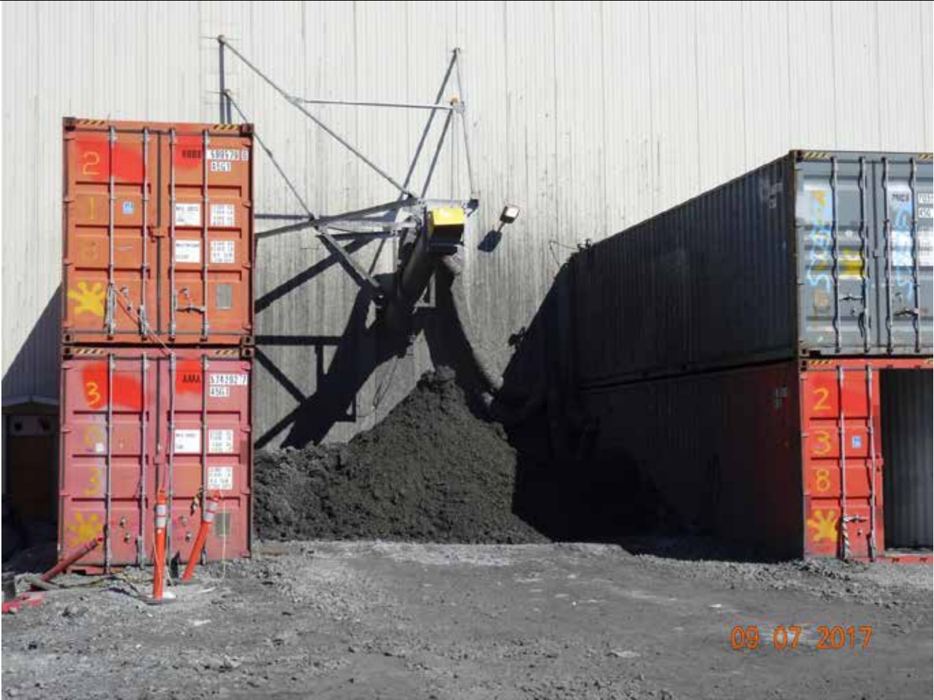
Description: Detoxified tailings are now deposited on the pad, and moved by excavator into trucks.
