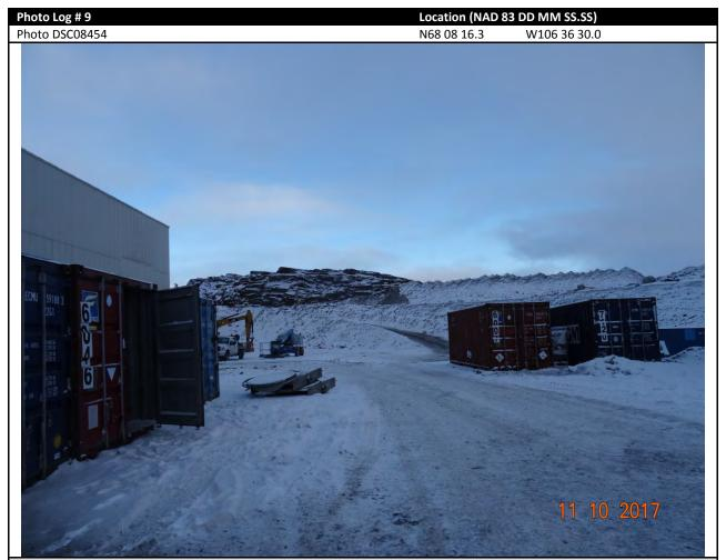
**Description:** Photo looking east with Mill to North. Shortcut now exists directly back to portal for trucks hauling waste underground, rather than traveling outside the 'contact area' where all contact water reports to the Sed and PC ponds.
