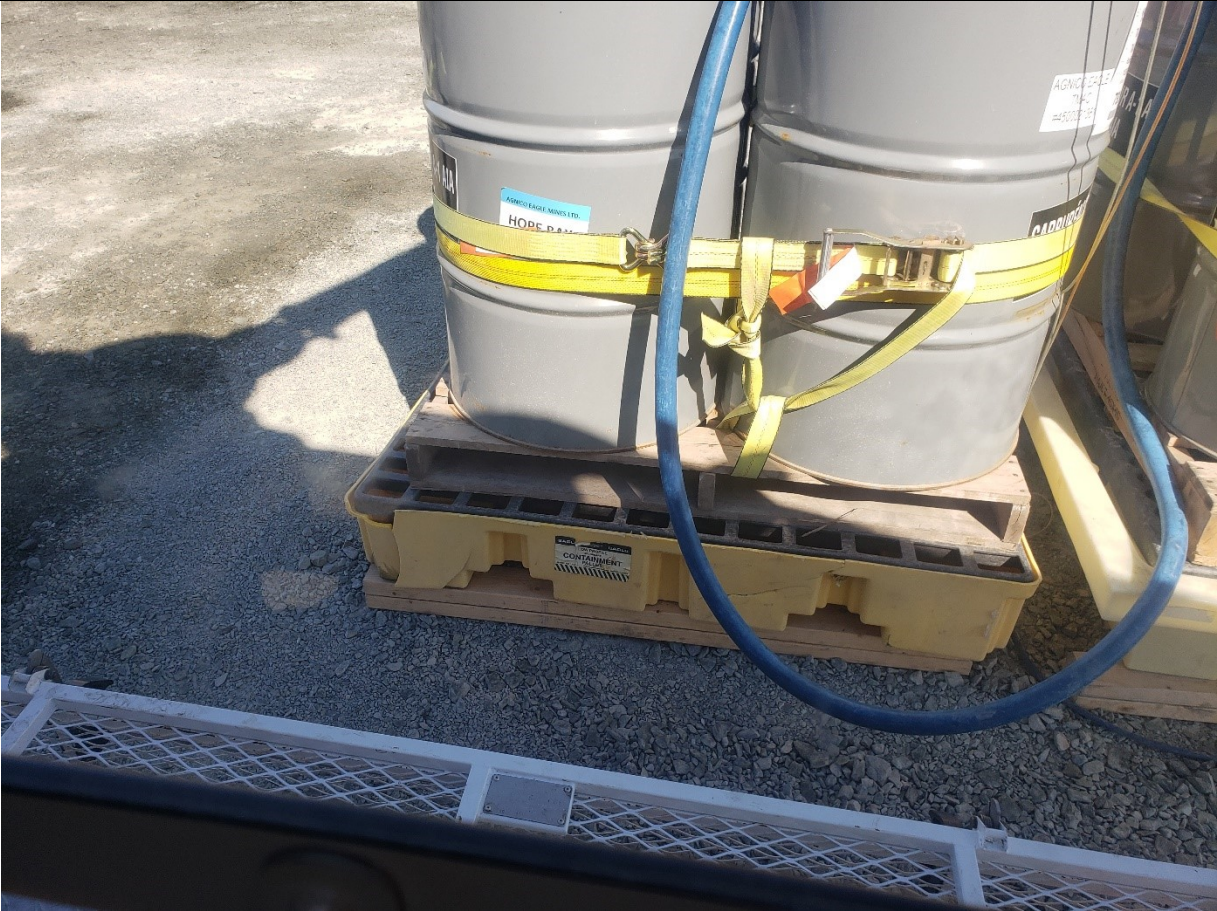
Description: Helicopter Pad fuel broken secondary containment.
