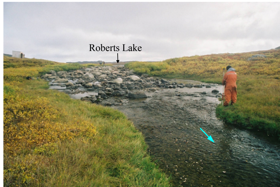
Plate 8 Roberts Outflow, 1 September 2002. Survey measurement of boulder garden to determine stream gradient.
