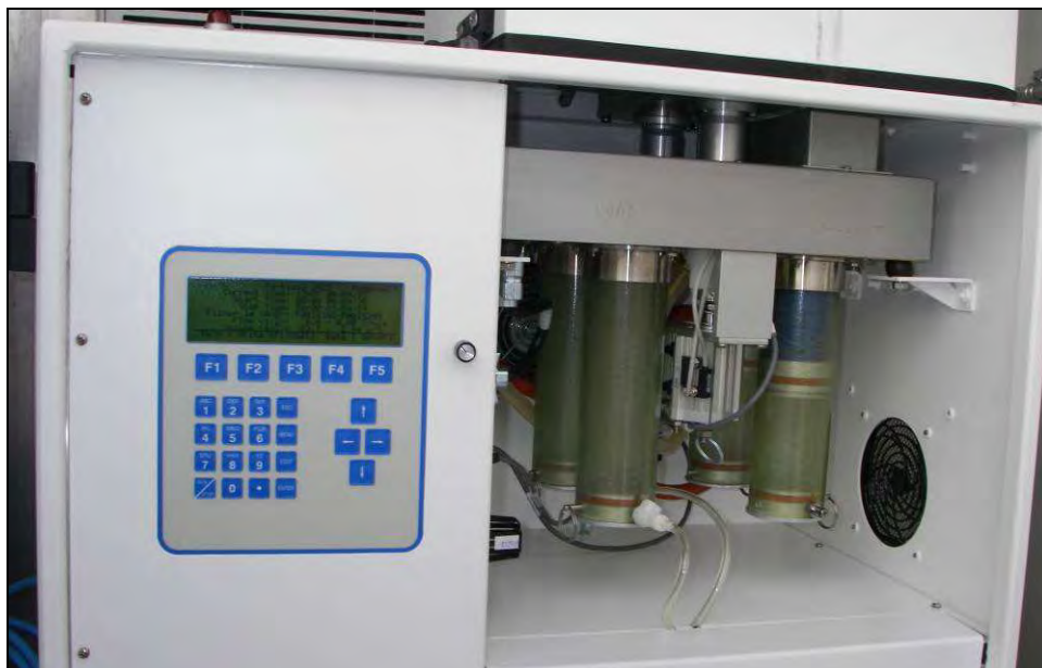
Plate 2.1-4. The Partisol air sampler filters are contained in a magazine on the left side of the unit. The filters laden with suspended particulate matter are contained in a magazine on the right side of the unit (PM 10 at front and PM 2.5 at rear).
