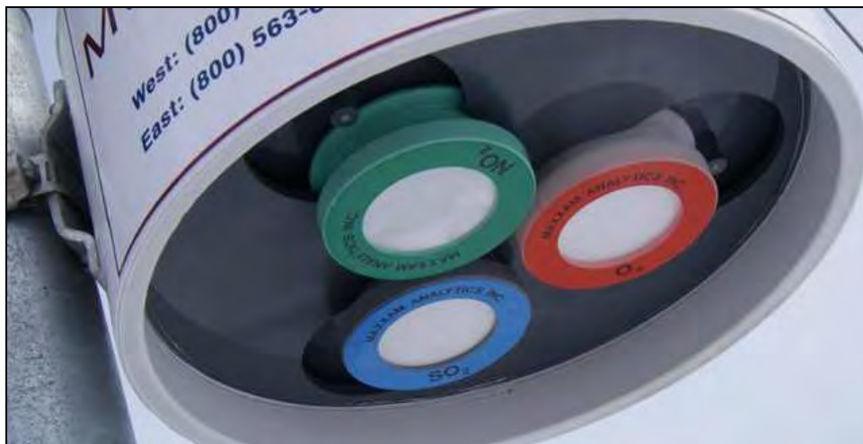
Plate 3.2-1. Passive air samplers under a rain shelter at Doris meteorological station.
