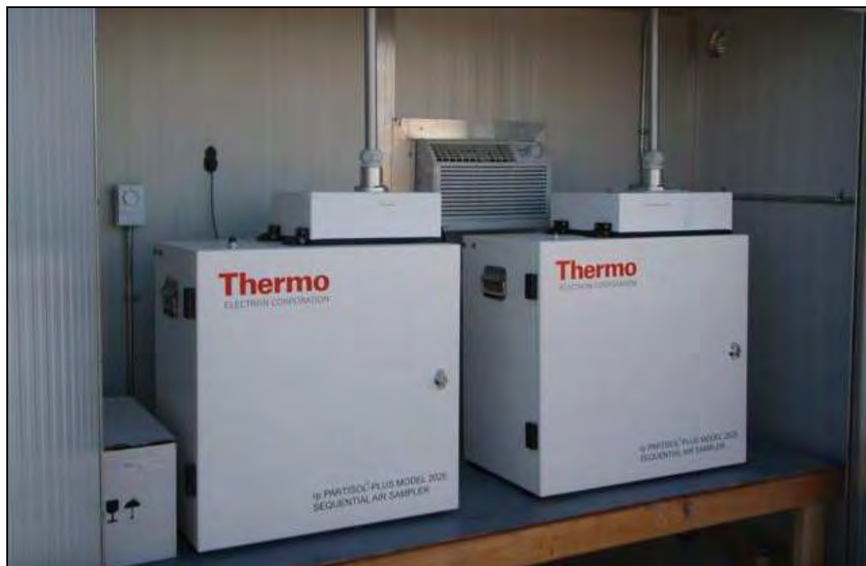
Plate 2.1-3. Inside the temperature controlled shelter the Partisol sampler which monitors TSP is shown on the left and the Partisol sampler which monitors PM_{10} and PM_{2.5} is on the right.
