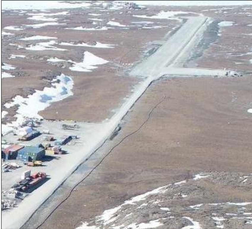
Photo 28: Showing pipeline alignment on the east side of the road and crossing on the west side before the airstrip.
