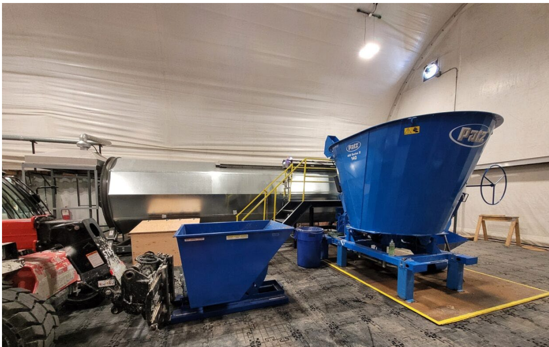
Photo 4: Brome 624A In-vessel Composter with Ventilation
