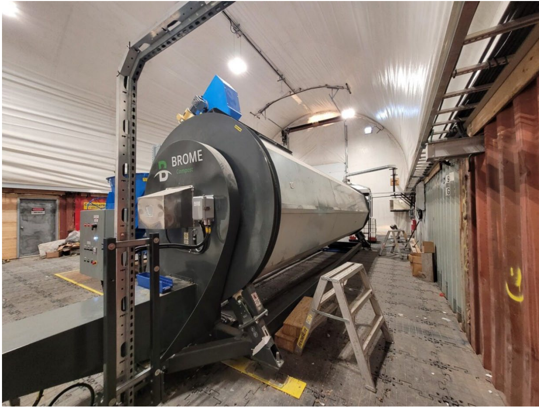
Photo 3: Brome 624A In-vessel Composter
