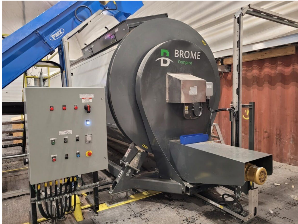
Photo 1: Brome 624A In-vessel Composter
