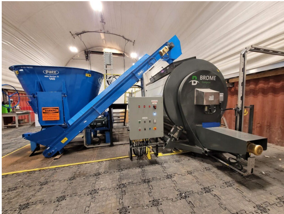
Photo 2: Brome 624A In-vessel Composter
