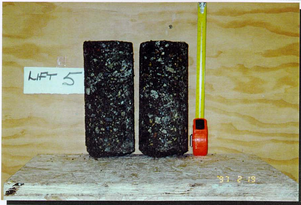
Photo 7 Typical Core Sample "Zone B" (97/02/19)
