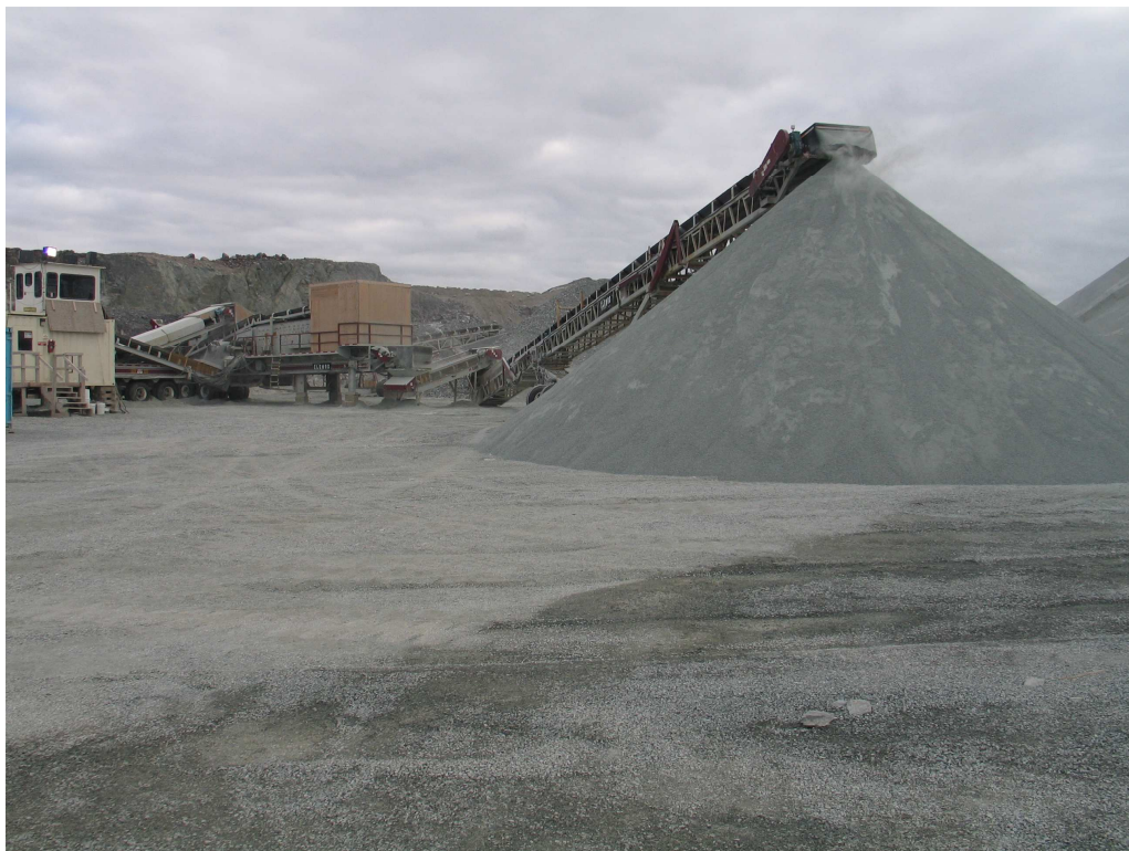
Photo 4: Stockpile of frozen core fines crushed from 5/8" clear.
